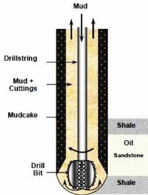
**Figure 1.5: Schematic diagram showing a drill string and bit**
