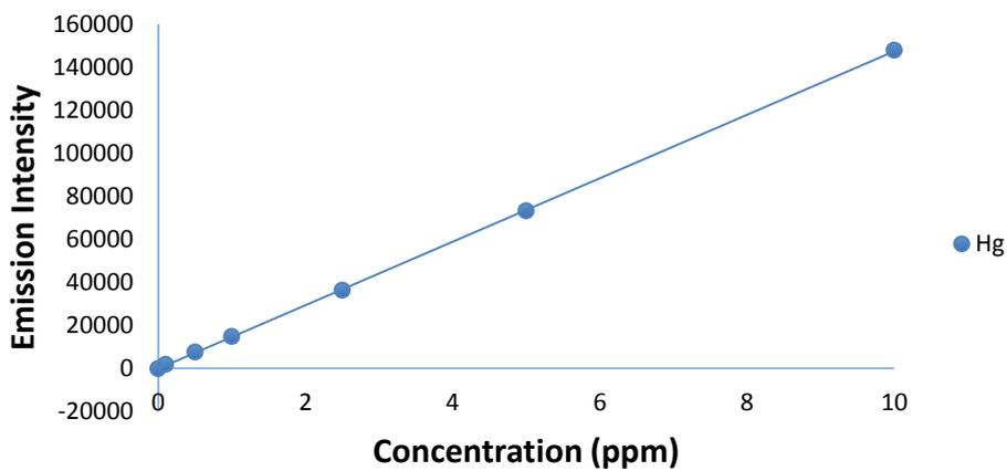
**Figure A.5: Calibration Plot for the Analysis of Hg in DCS by ICP-OES**
