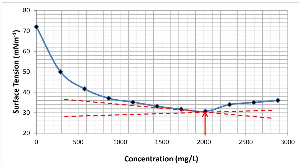
**Figure 3.20: Determination of CMC of Sodium Dodecyl Sulphate (SDS)**
