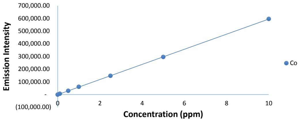
**Figure A.10: Calibration Plot for the Analysis of Co in DCS by ICP-OES**
