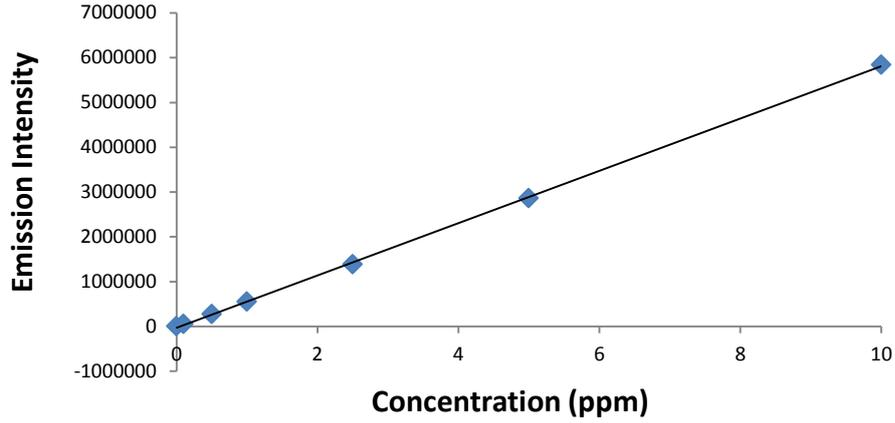
**Figure 2.11: Calibration Plot for the Analysis of Al in DCS by ICP-OES**
