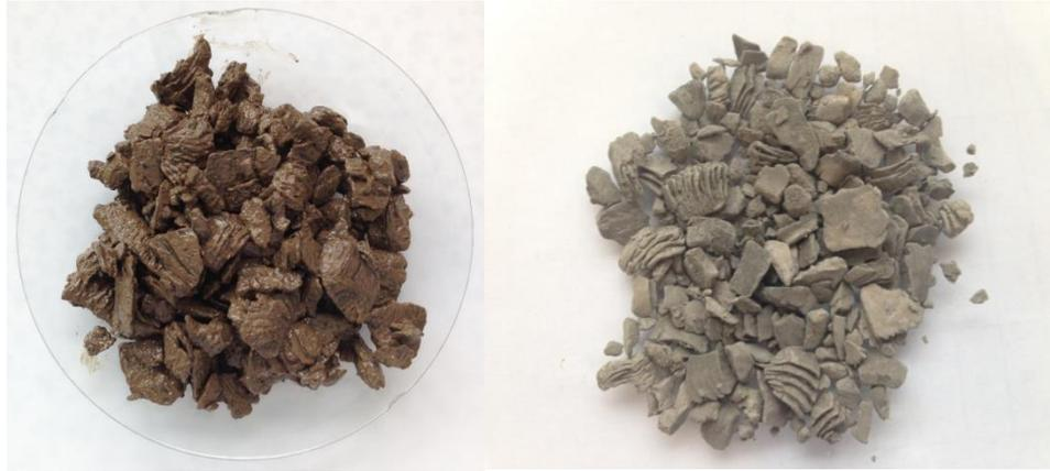
**Figure 2.4: Oil Based Mud Drill Cuttings:**
