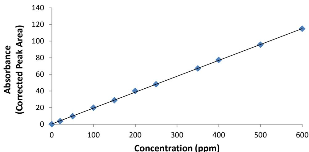
**Figure 2.17: FT-IR Calibration Curve for Diesel in Perklone.**
