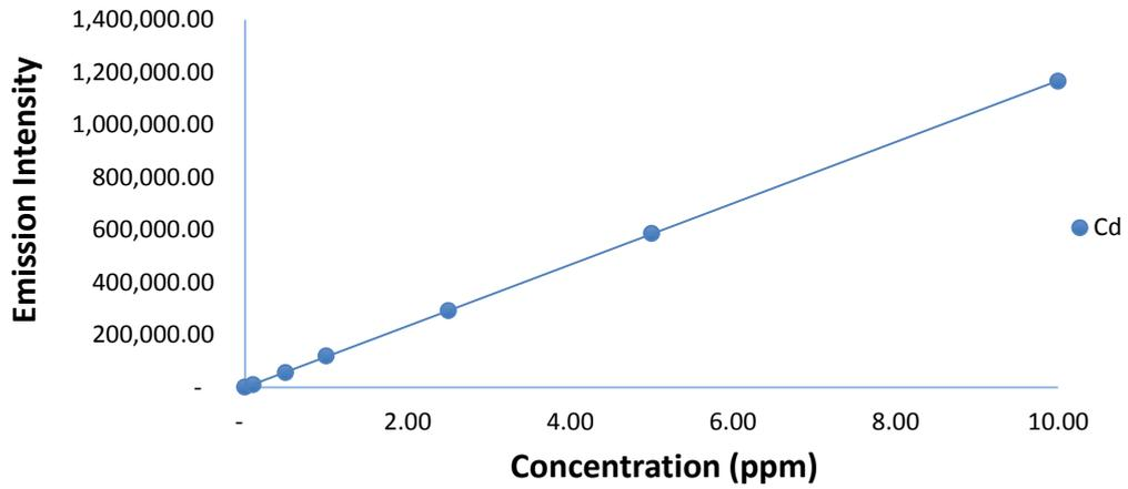
**Figure A.7: Calibration Plot for the Analysis of Cd in DCS by ICP-OES**
