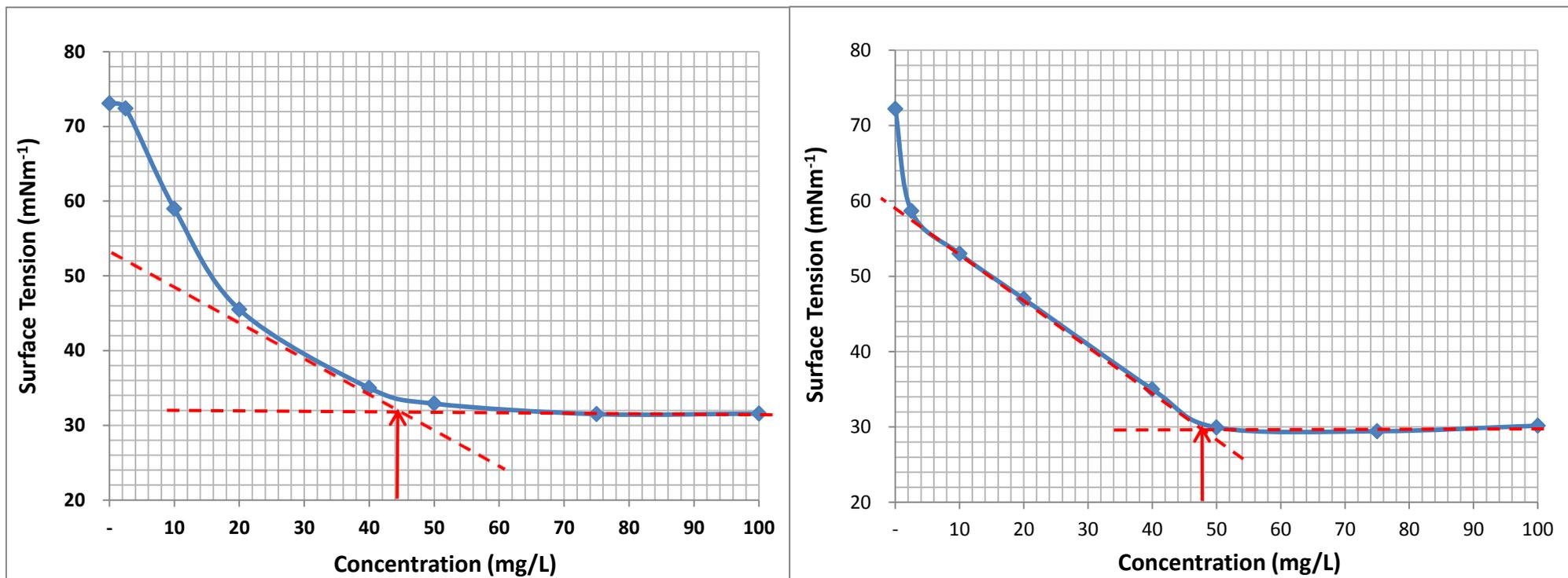
**Figure 3.21: Determination of CMC of Crude Rhamnolipid, Produced from *Ps. aeruginosa* sp.**
