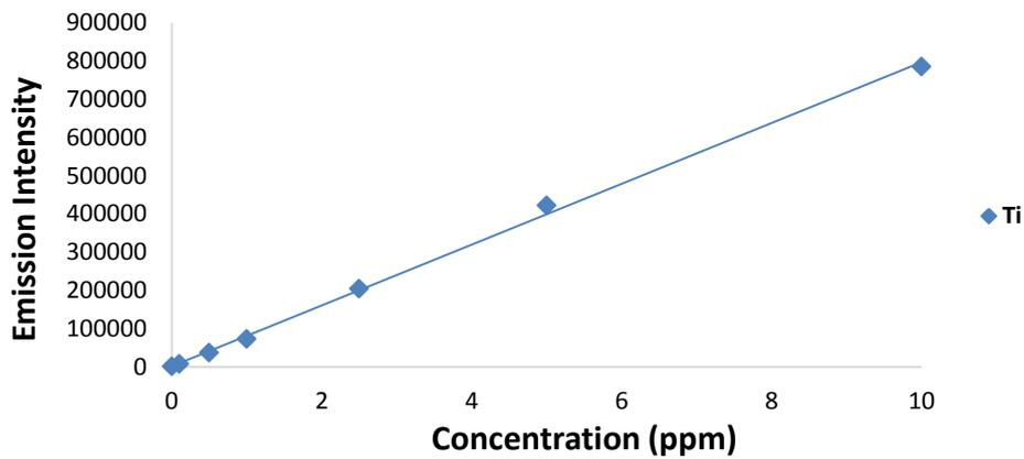
**Figure A.1: Calibration Plot for the Analysis of Ti in DCS by ICP-OES**
