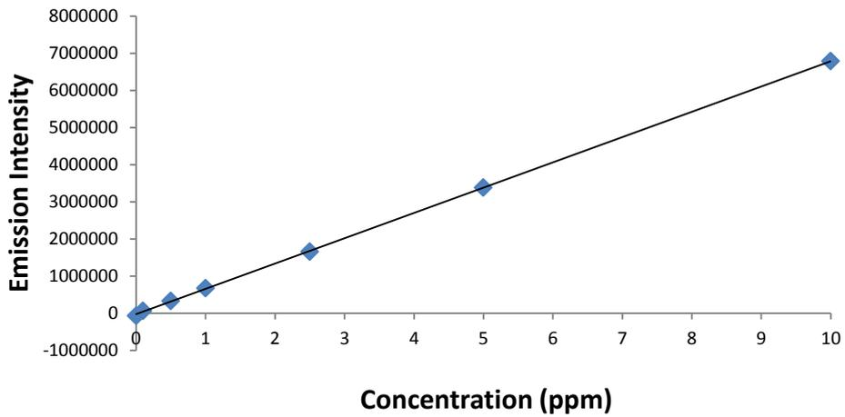
**Figure 2.12: Calibration Curve for the Analysis of Mg in DCS by ICP-OES**
