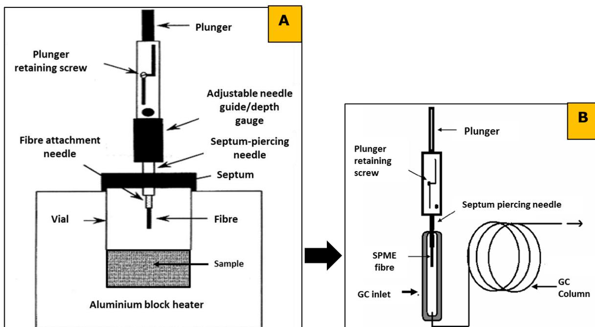
**Figure 2.2: Schematic diagram of a HS-SPME system**
