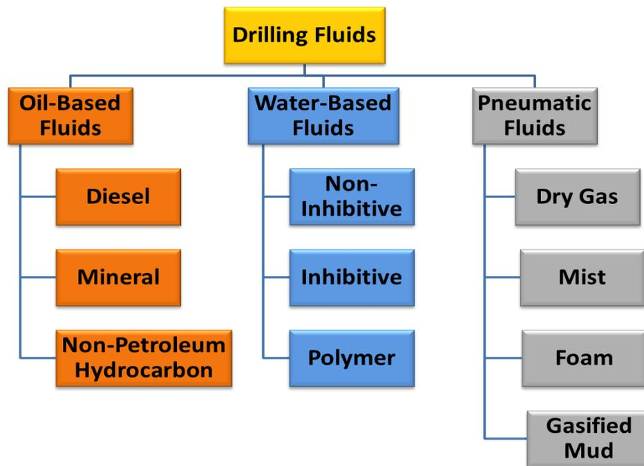
**Figure 1.7: Drilling Fluid Classification**
