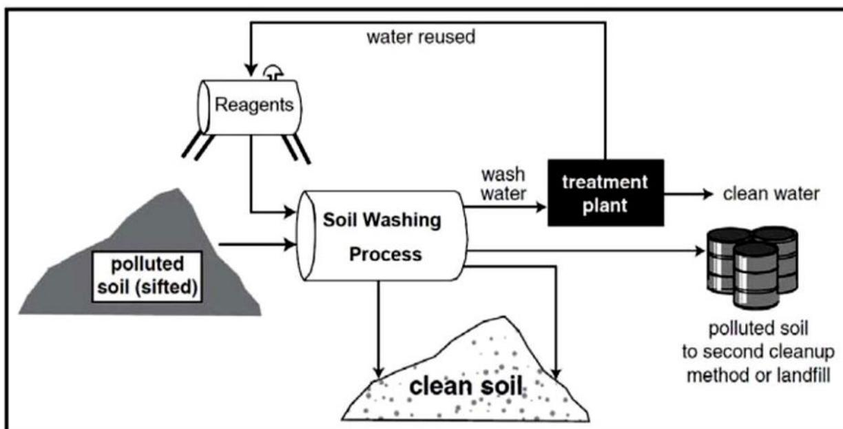
**Figure 4.2: Schematic diagram of a Typical Soil Washing Process**
