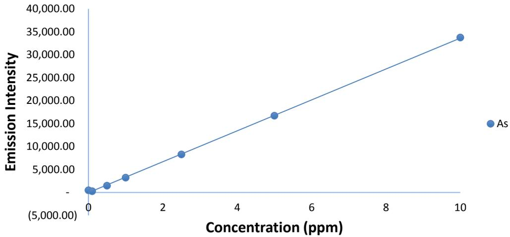
**Figure A.13: Calibration Plot for the Analysis of As in DCS by ICP-OES**
