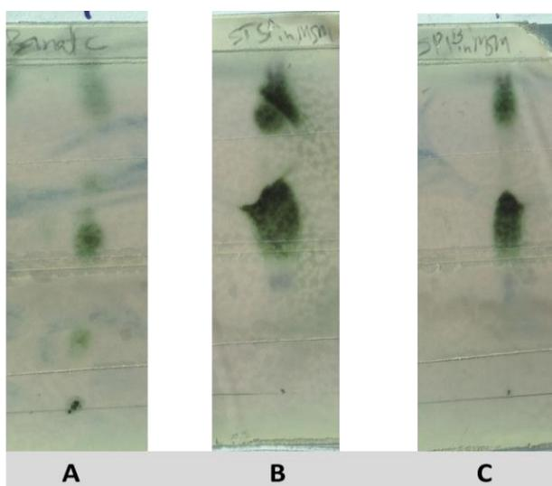
**Figure 3.17: Thin Layer Chromatography of Rhamnolipids using Anisaldehyde Reagent (Sugar Test)**
