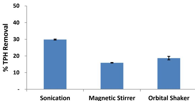
**Figure 2.18: TPH Extraction Methods**
