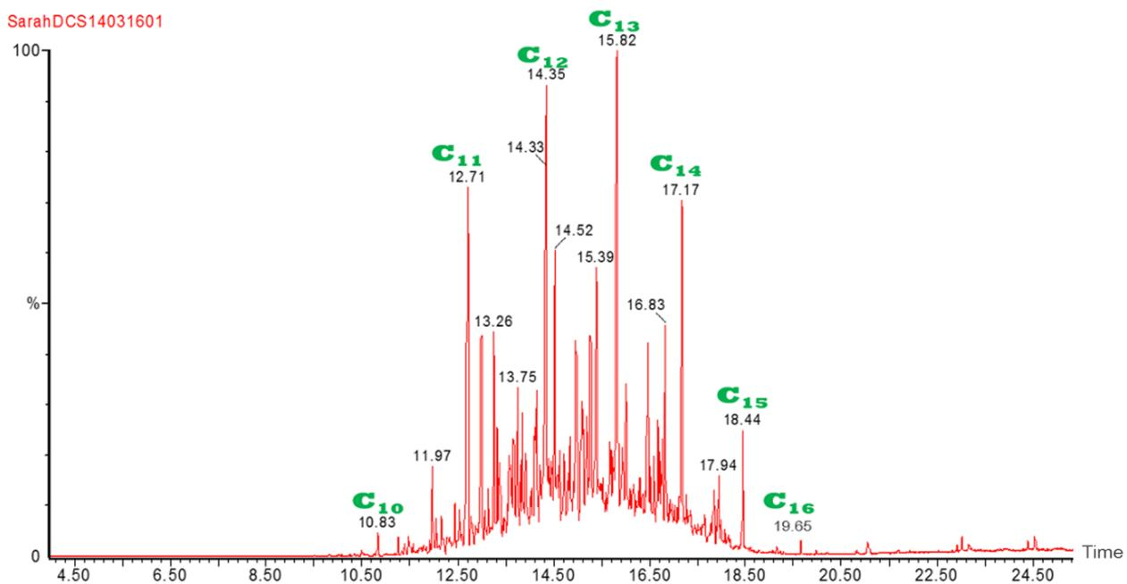
**Figure 2.14: Total Ion Chromatogram of OBM Drill Cuttings**
