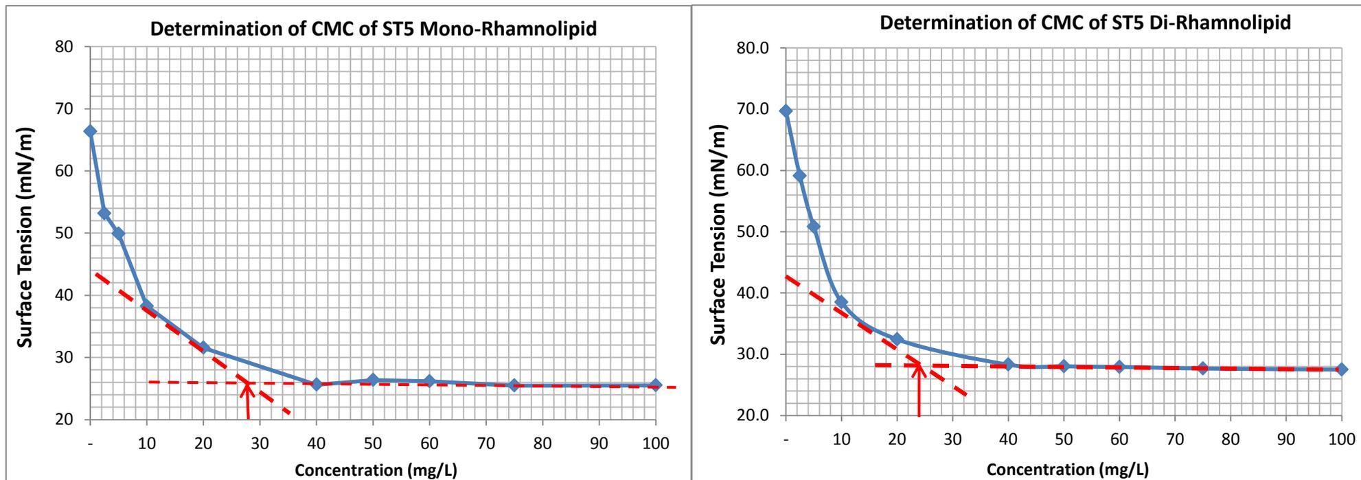
**Figure 3.22: Determination of CMC of Purified Rhamnolipid Produce from *Ps. Aeruginosa* ST5**
