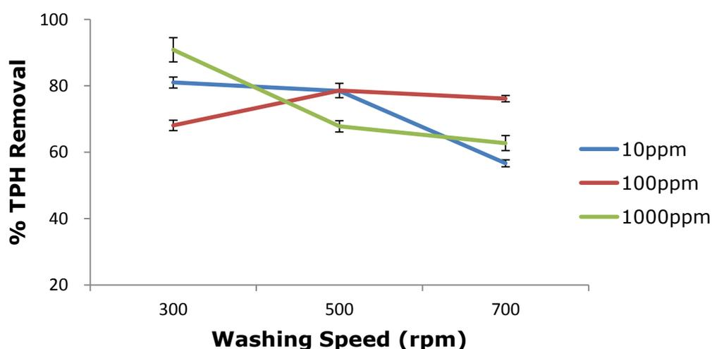
**Figure 4.9: Effect of Washing Speed on TPH Removal**
