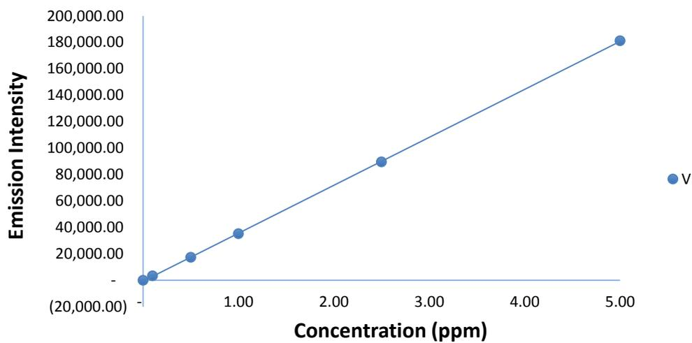
**Figure A.6: Calibration Plot for the Analysis of V in DCS by ICP-OES**
