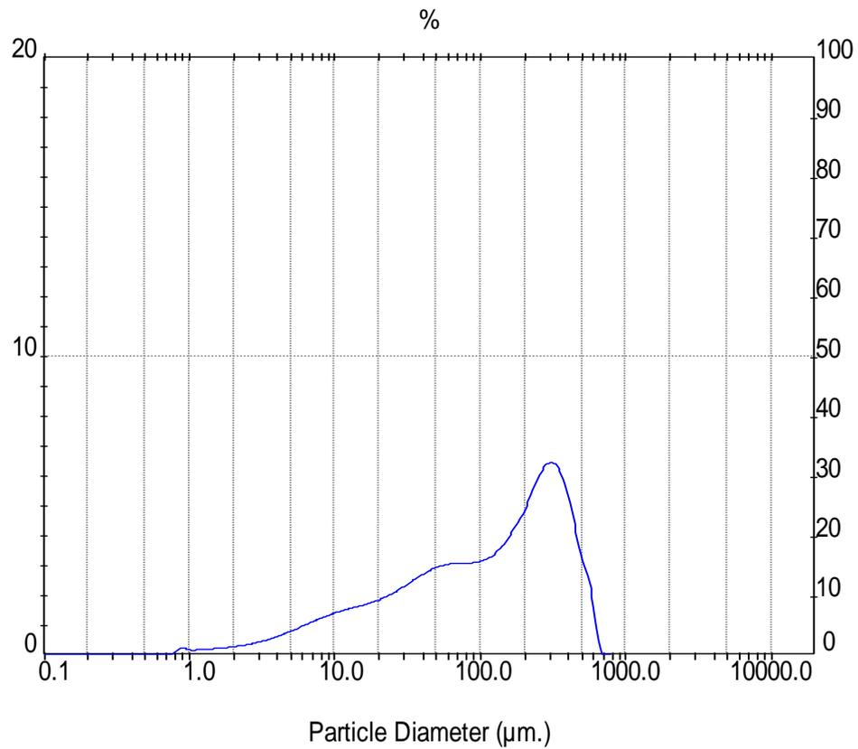
**Figure 2.5: Particle Size Distribution (PSD) of Soil by Laser Diffraction Analysis**
