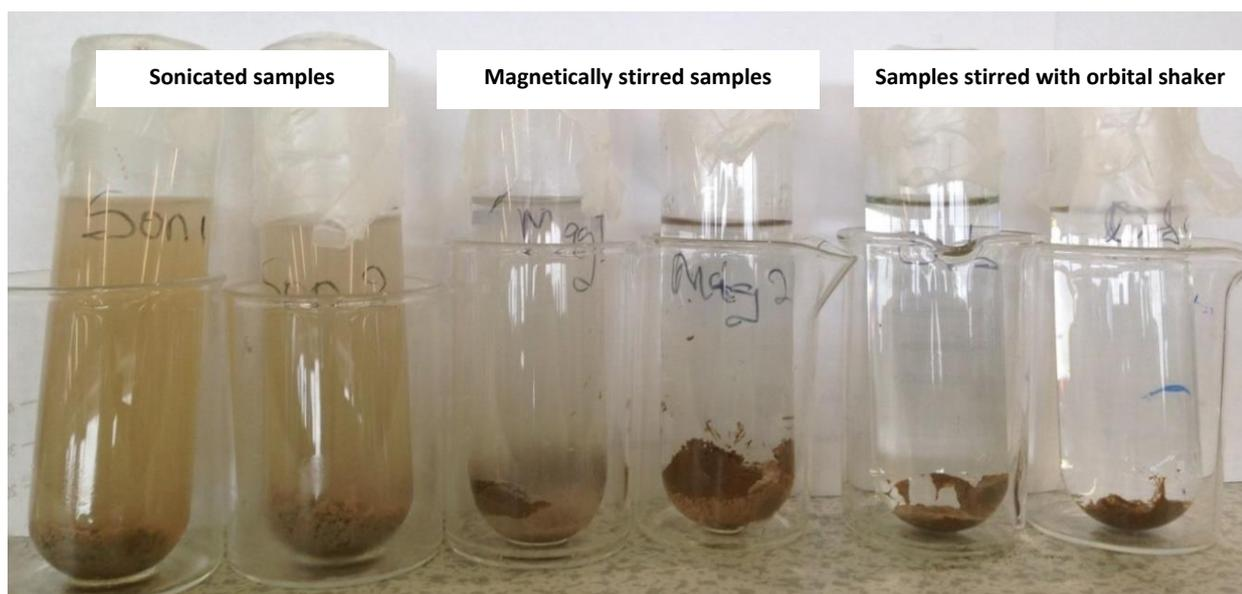
**Figure 2.3: Determination of TPH Extraction Method from Contaminated Solids**
