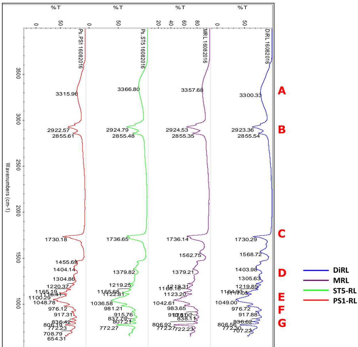
**Figure A.16: FTIR Spectra for Rhamnolipids** (DiRL, MRL, ST5-RL and PS1-RL).
