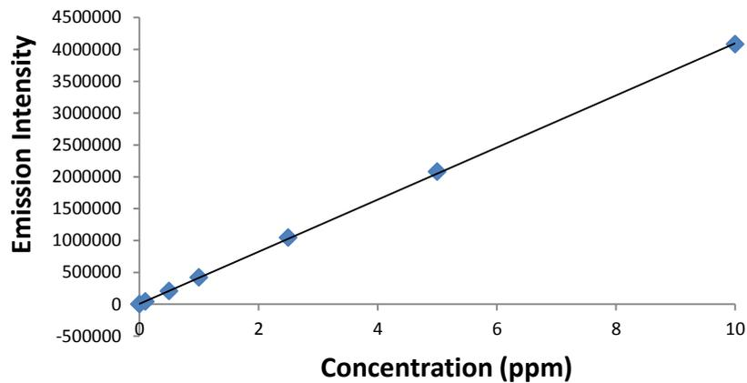
**Figure 2.13: Calibration Curve for the Analysis of Ba in DCS by ICP-OES**
