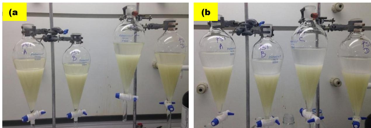
**Figure 3.9: Solvent extraction of rhamnolipid using ethyl acetate.**
