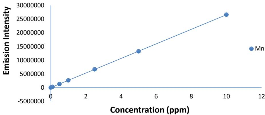
**Figure A.2: Calibration Plot for the Analysis of Mn in DCS by ICP-OES**
