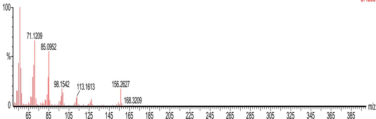
**Figure 2.16: Mass Spectra of Undecane (C<sub>11</sub>H<sub>24</sub>), @12.71 minutes**
