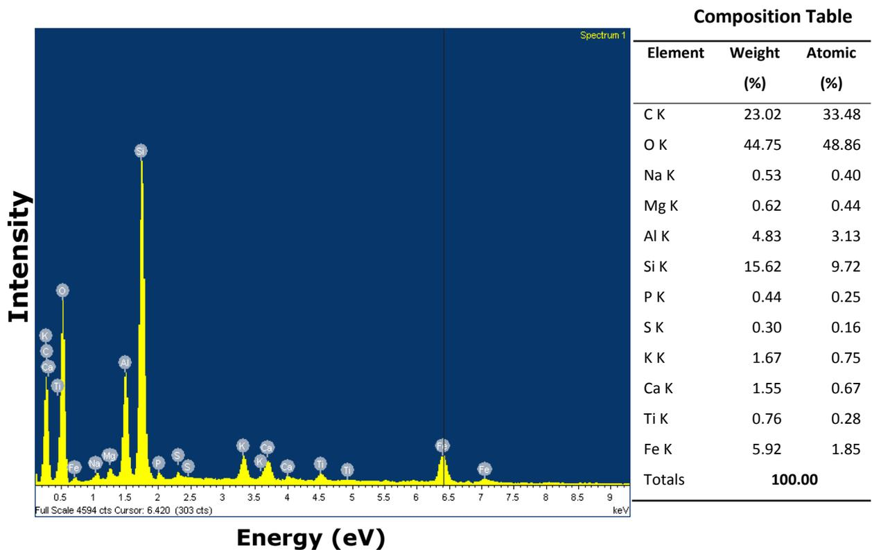
**Figure 2.10: An SEM-EDX Spectrum of Soil Samples – As Received**
