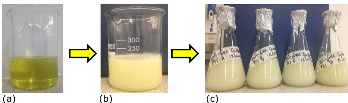
**Figure 3.8: Removal of Bacteria Cells for the Recovery of Biosurfactant**
