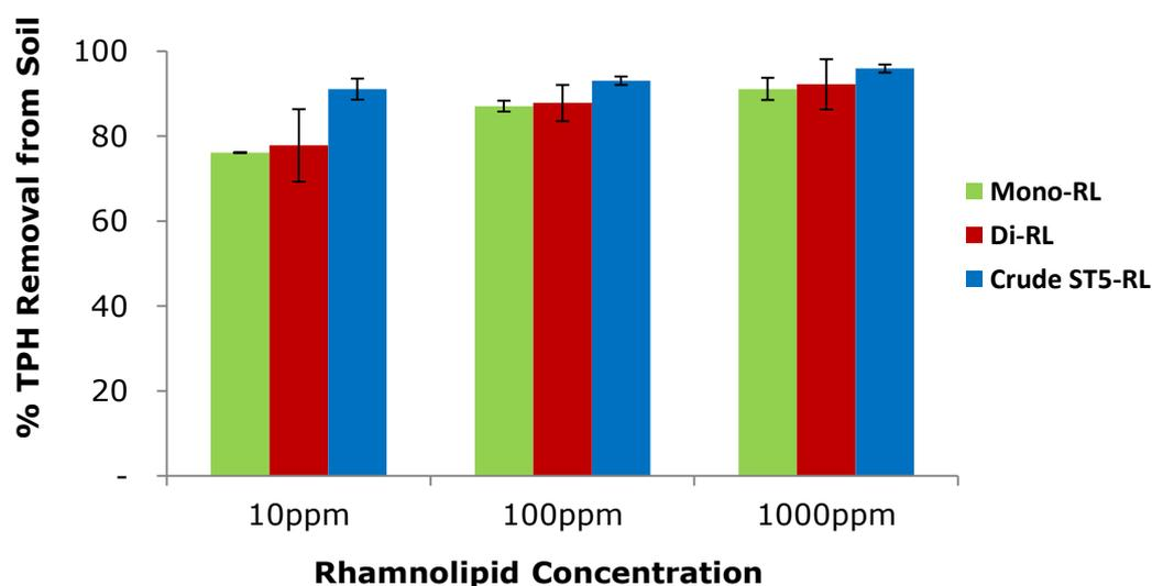
**Figure 4.6: Performance of Biosurfactants in TPH Removal from Oil Contaminated Soil**
