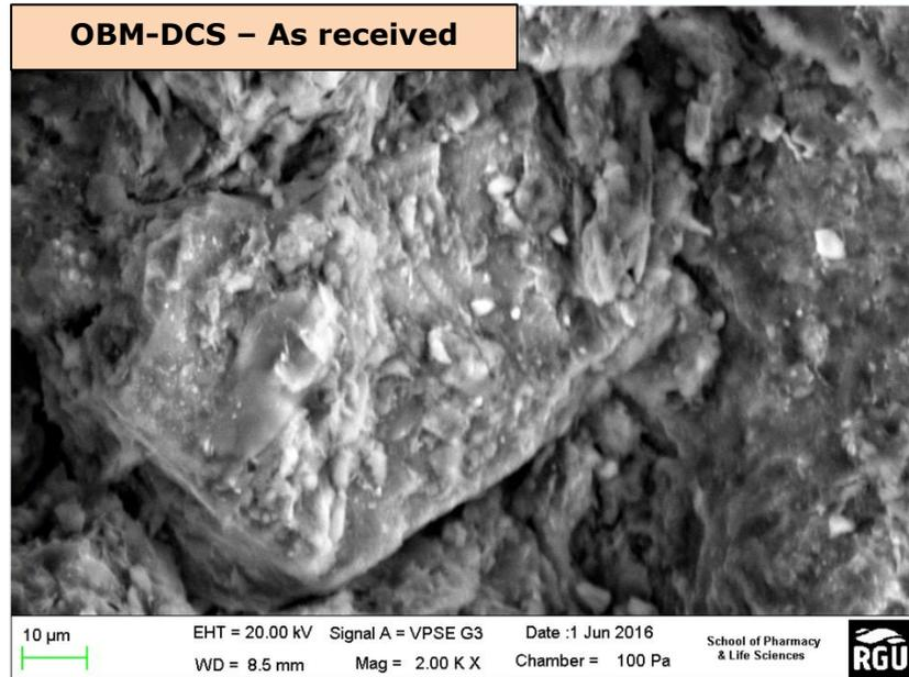
**Figure 2.7: Microstructure of OBM Drill Cuttings at 2000X Magnification**
