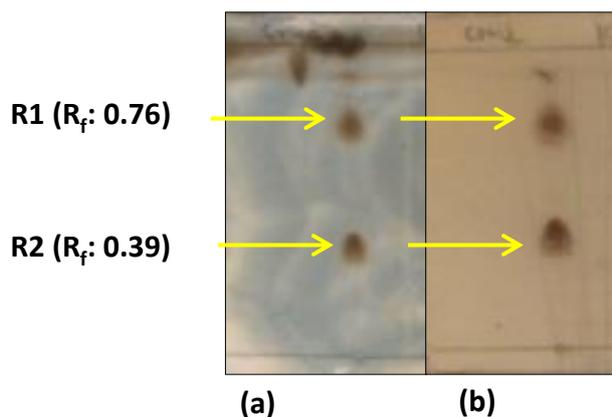
**Figure 3.19: Thin Layer Chromatography of Crude ST5 Rhamnolipid**
