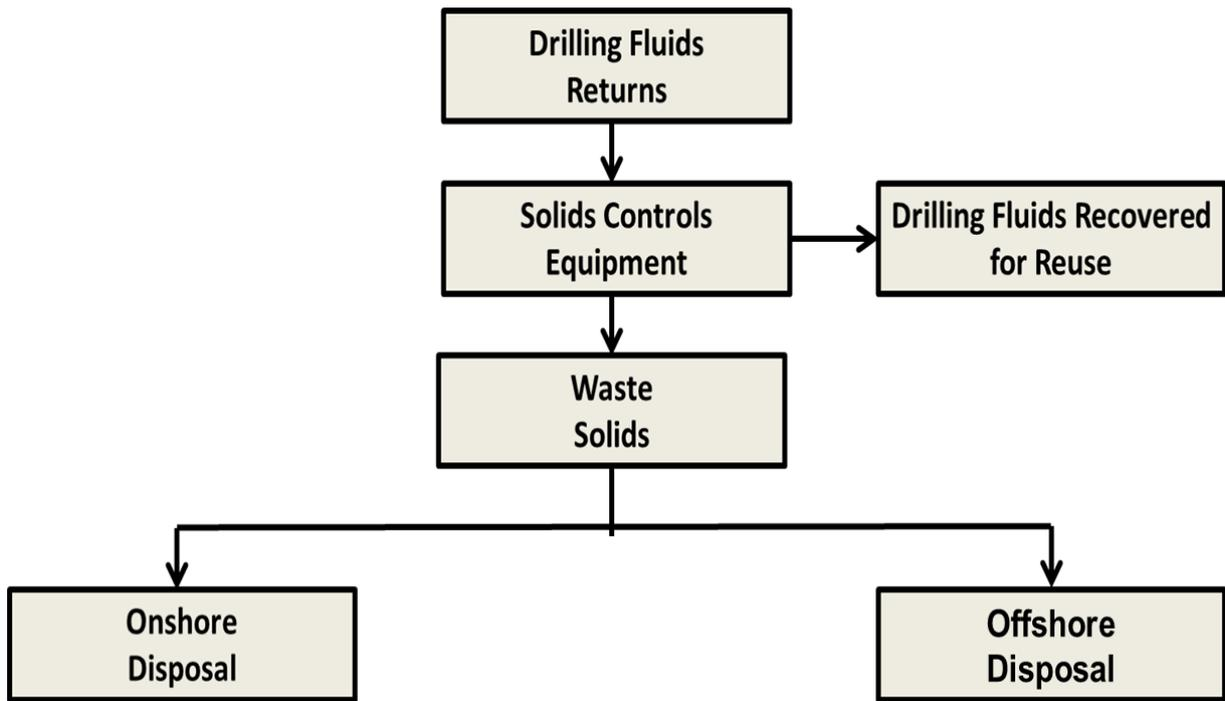
**Figure 1.9: Schematic Flow Chart Showing Separation of Drill Cuttings from Drilling Fluids Solid Waste Disposal Options**
