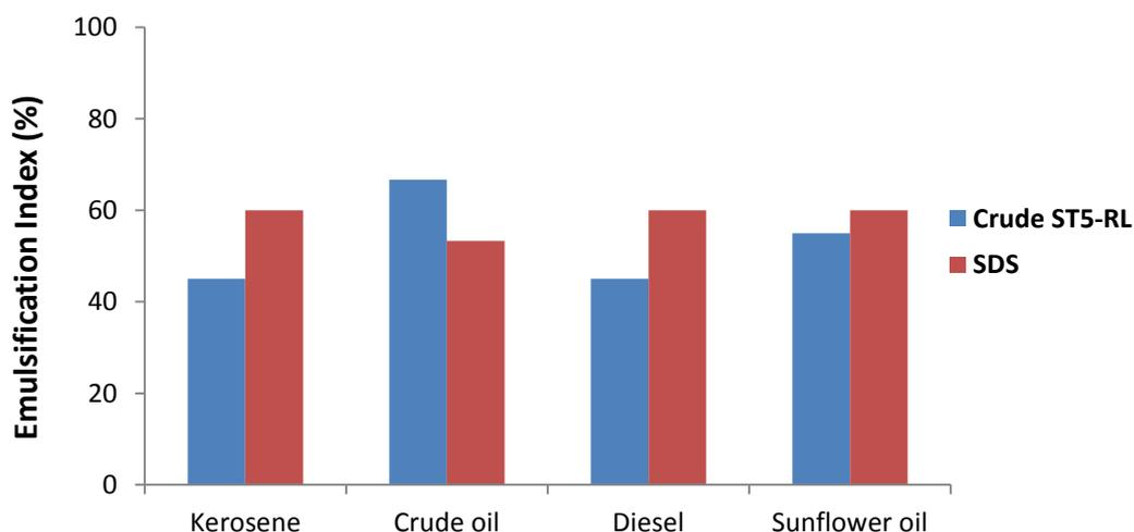
**Figure 3.23: Emulsification Activity of SDS and Crude ST5 Rhamnolipid on Selected Oils**
