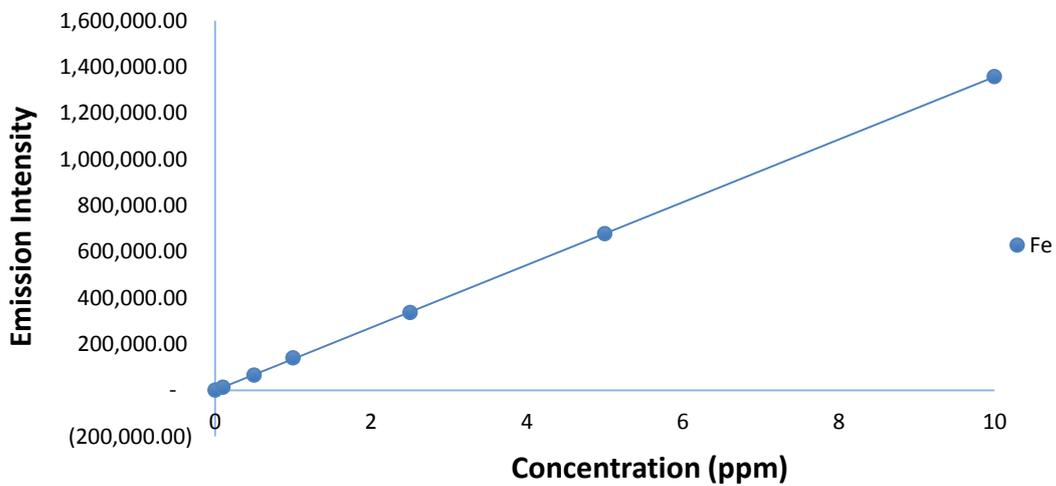
**Figure A.11: Calibration Plot for the Analysis of Fe in DCS by ICP-OES**
