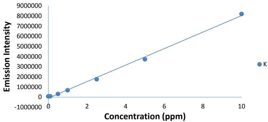
**Figure A.4: Calibration Plot for the Analysis of K in DCS by ICP-OES**
