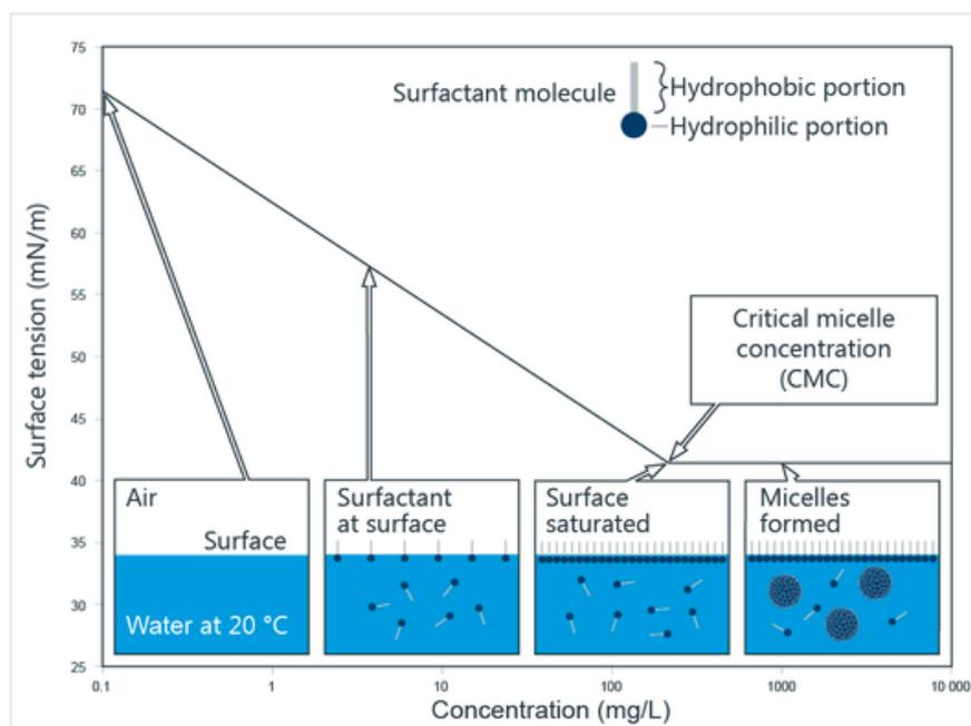
**Figure 3.11: Typical Plot for the Determination of CMC by Tensiometry**
