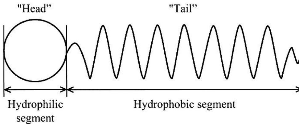
**Figure 3.1: Structure of a Typical Surfactant**
