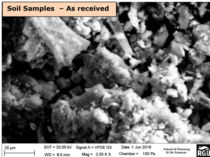
**Figure 2.8: Microstructure of Soil Sample at 2000X Magnification**
