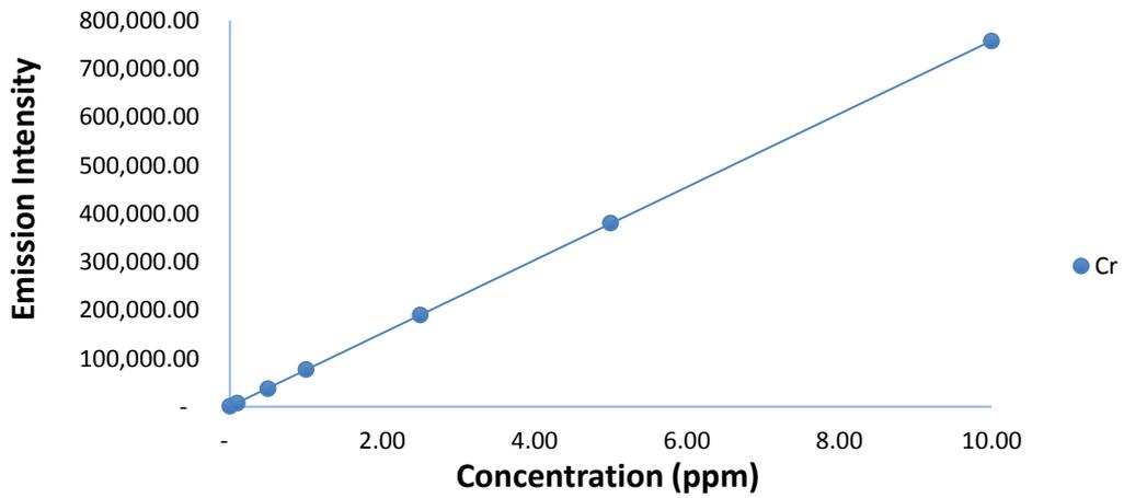
**Figure A.8: Calibration Plot for the Analysis of Cr in DCS by ICP-OES**
