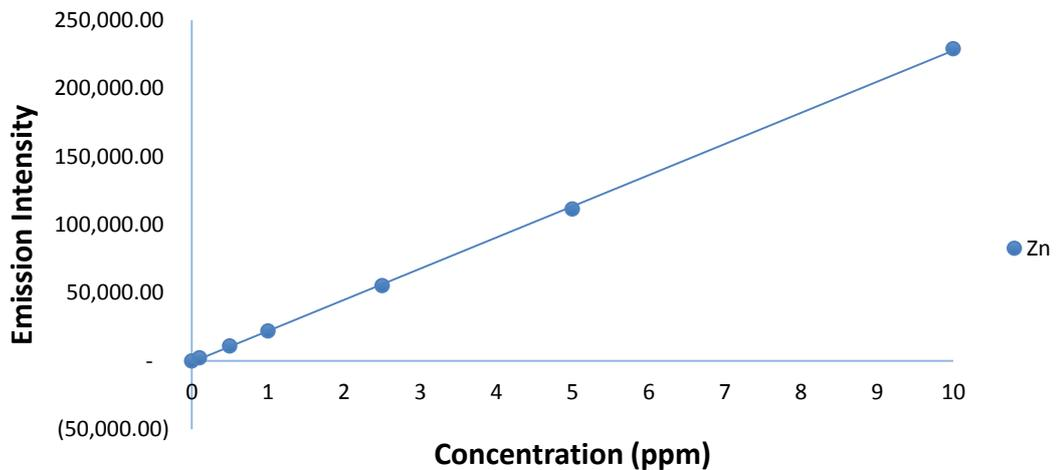
**Figure A.15: Calibration Plot for the Analysis of Zn in DCS by ICP-OES**
