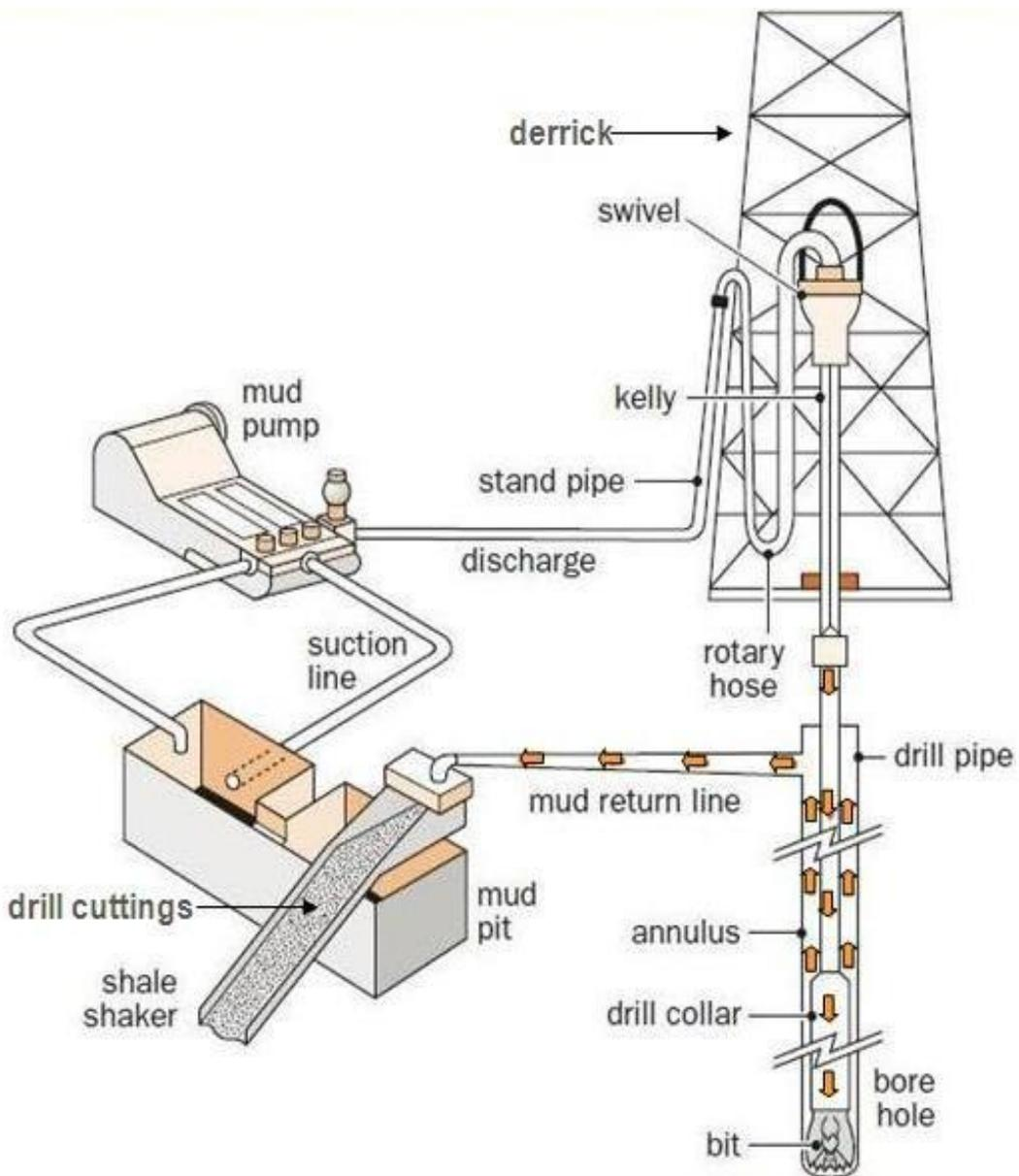
**Figure 1.4: A Schematic Diagram of a Drilling Mud Circulation System**
