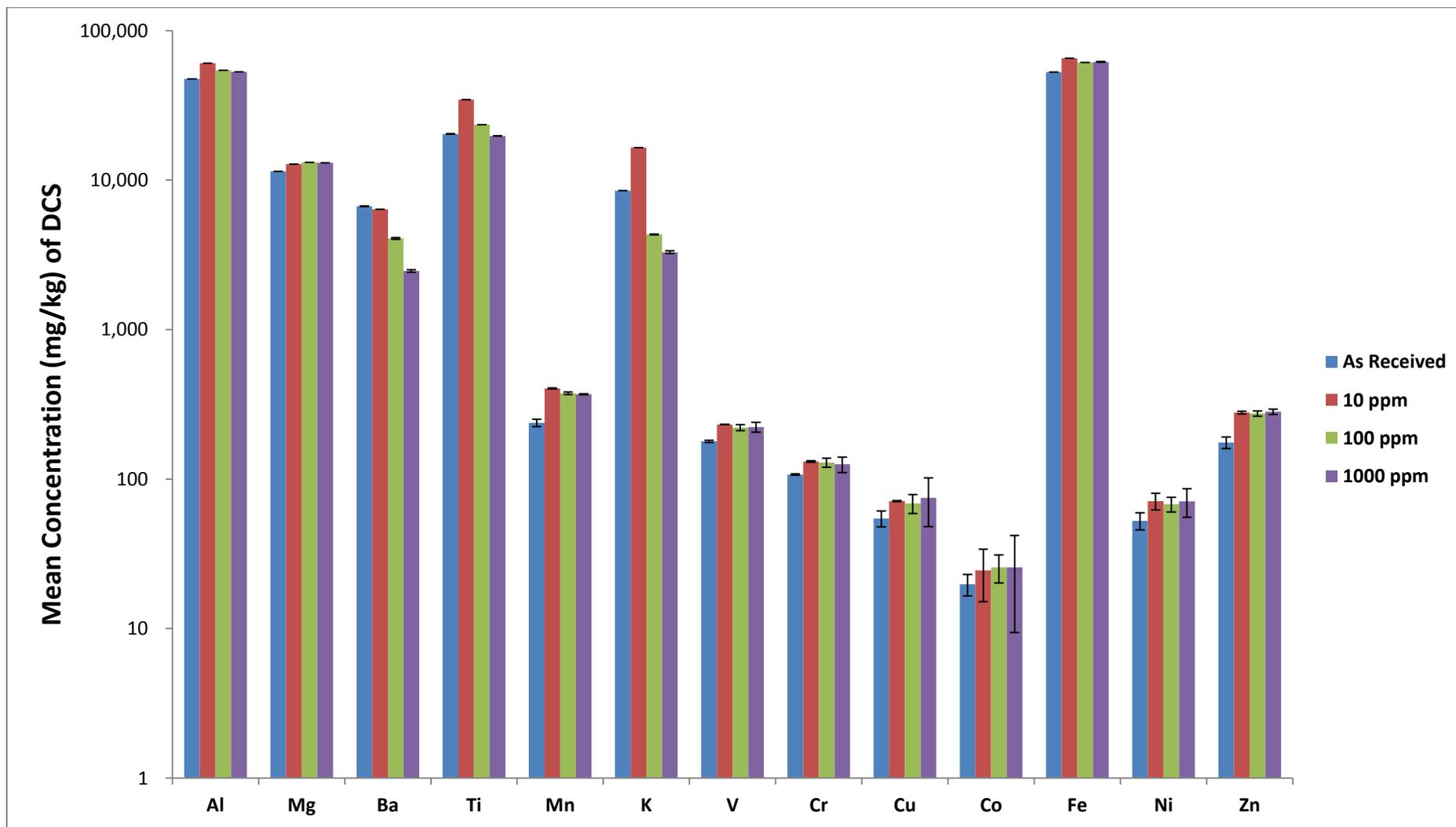
**Figure 4.16: Elemental Content by ICP-OES of OBM-DCS as received and following Crude ST5 Rhamnolipid Washing (n=2)**
