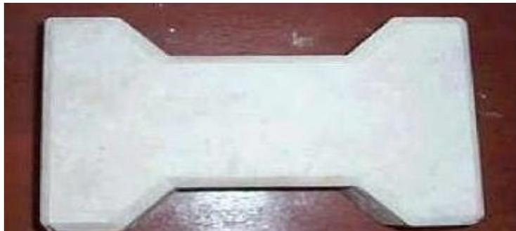
**Figure 1.10: Interlocking Bricks Produced with DCR Treated Drill Cuttings.**
