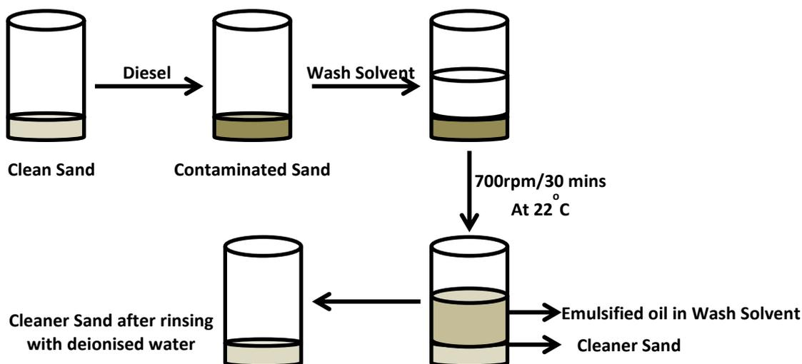
**Figure 4.3: Schematic Diagram of the Sand Washing Process**
