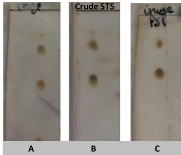
**Figure 3.18: Thin Layer Chromatography of Rhamnolipids using Ceric Ammonium Molybdate Reagent (Lipid Test)**
