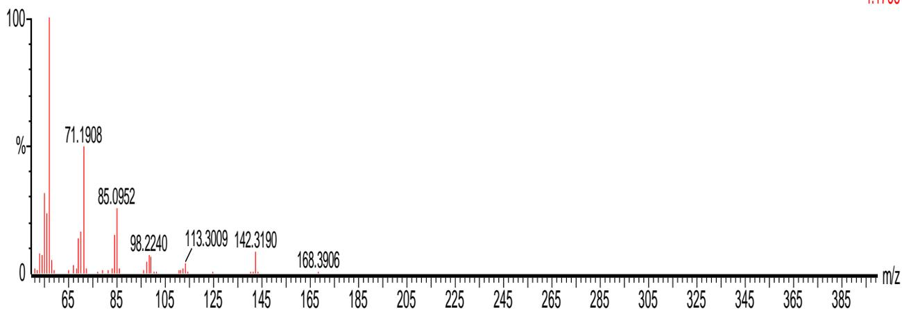
**Figure 2.15: Mass Spectra of Decane (C<sub>10</sub>H<sub>22</sub>), @10.83 minutes**
