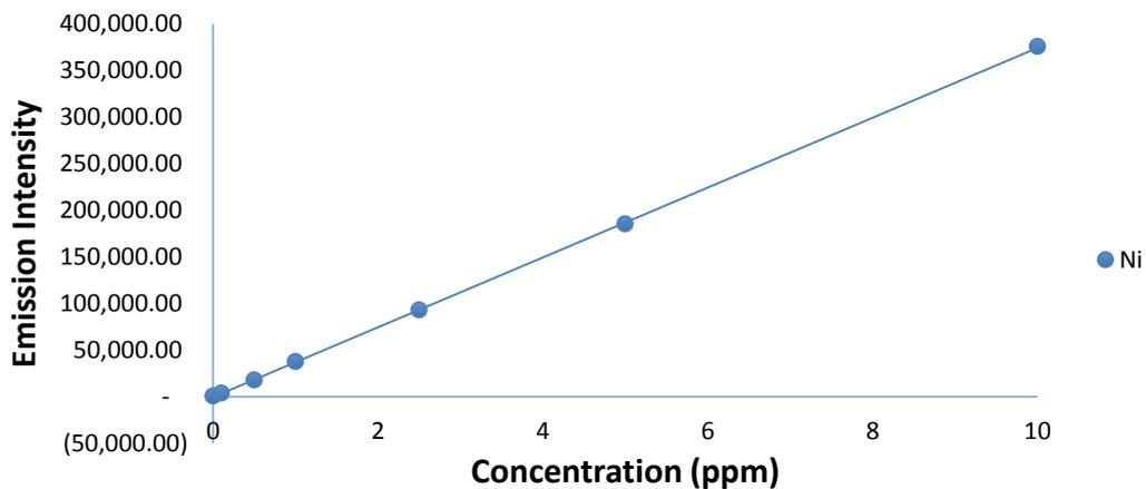
**Figure A.12: Calibration Plot for the Analysis of Ni in DCS by ICP-OES**
