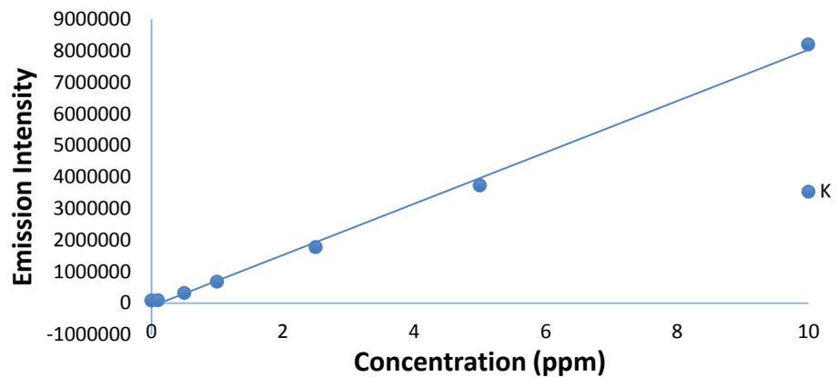
**Figure A.3: Calibration Plot for the Analysis of K in DCS by ICP-OES**
