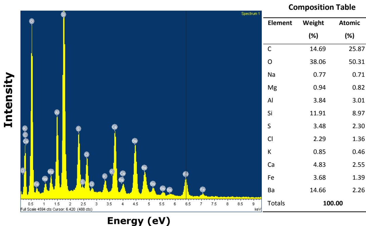
Figure 2.9: A SEM-EDX Spectrum of OBM-DCS – As received
