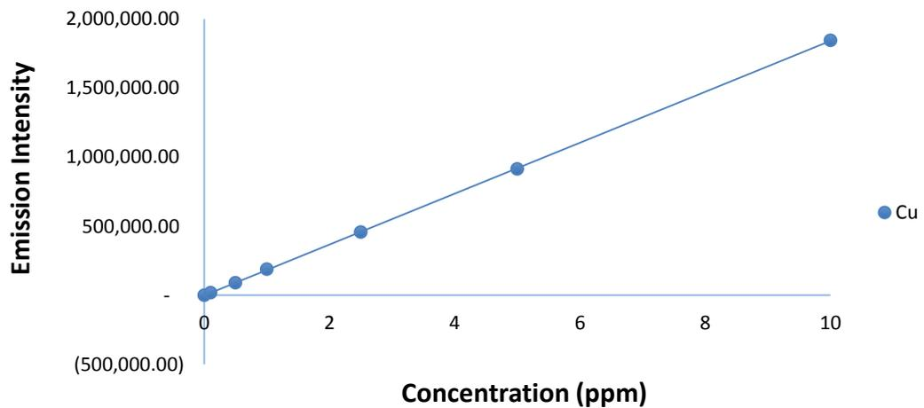
**Figure A.9: Calibration Plot for the Analysis of Cu in DCS by ICP-OES**
