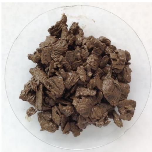
**Figure 2.1: Oil Based Mud (OBM) Drill Cuttings As Received**
