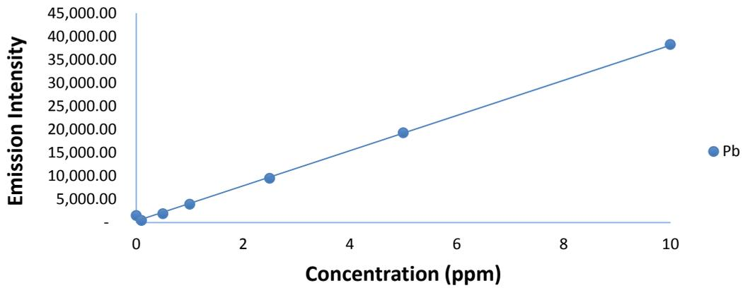
**Figure A.14: Calibration Plot for the Analysis of Pb in DCS by ICP-OES**
