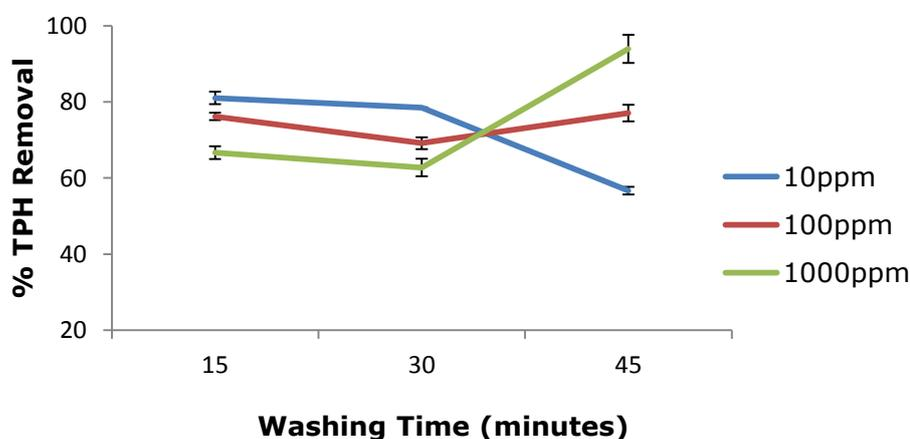
**Figure 4.8: Effect of Washing Time on TPH Removal**
