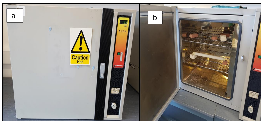
Figure 32: Oven drying of the membrane at 65°C (a) Picture of the oven showing the operating temperature, (b) Picture showing the membrane placed inside the oven for drying
