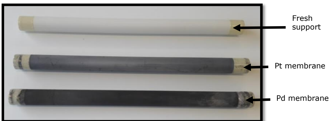
Figure 41: Picture showing the fresh support and activated platinum and palladium membranes
