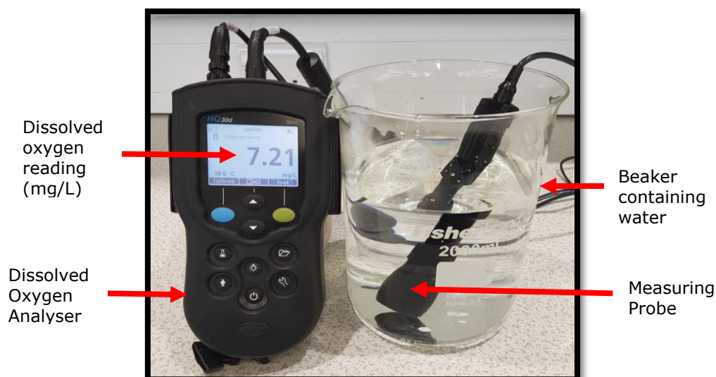
Figure 66: Process showing measuring of DO level in water
