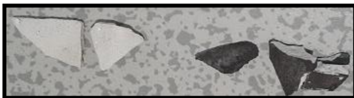
Figure 44: Picture showing fragments of the witness samples going in for SEM-EDAX analysis
