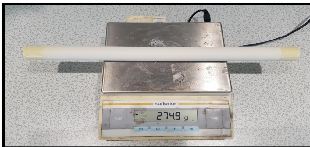
Figure 27: Picture showing the weighing of a ceramic support
