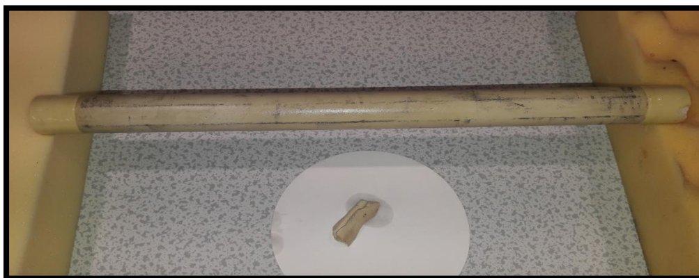
Figure 31: Air drying of the membrane at room temperature
