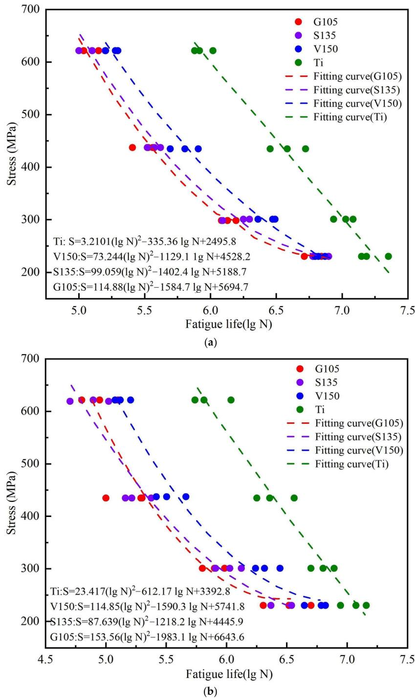
**Figure 3.** Fatigue curves of different drill pipe samples in H<sub>2</sub>S mud (a) at room temperature and (b) at 100 °C (adapted from [37]).
