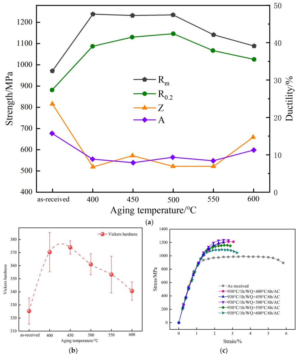
**Figure 1.** Effect of aging treatment on mechanical properties of Ti-5Al-3V-1.5Mo-2Zr titanium alloy drill pipe: (a) tensile property curve, (b) hardness change, (c) stress–strain curve (adapted from [21]).
