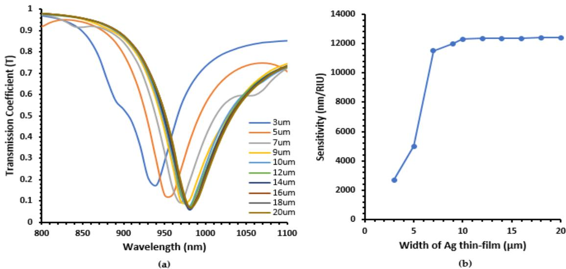
**Figure 4.** (a) Transmission spectra at RI = 1.42 and specific Ag widths; (b) Graph of sensitivity against specific Ag thin film widths of analyte RI from 1.41 to 1.42.
