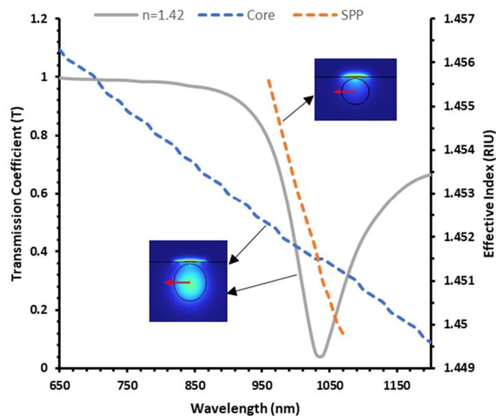
Figure 2. Phase matching between core and SPP mode of D-shaped sensor.
