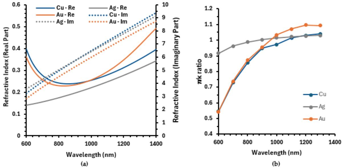
**Figure 6.** Graph of (a) real and imaginary refractive index against wavelength; (b)  $n/k$  against wavelength
