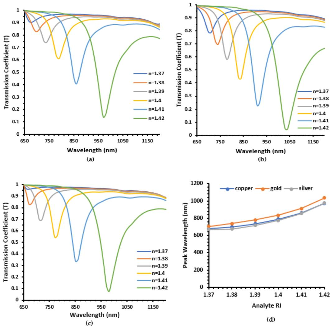
**Figure 5.** Transmission spectrum for (a) copper; (b) gold; (c) silver; (d) Peak wavelength as a function of analyte RI from 1.37 to 1.42.
