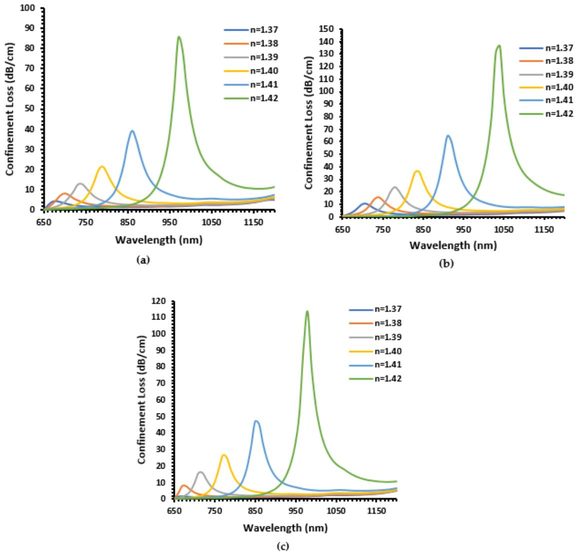
**Figure 7.** Confinement loss spectra for (a) copper; (b) gold; (c) silver thin film D-SPR sensor.
