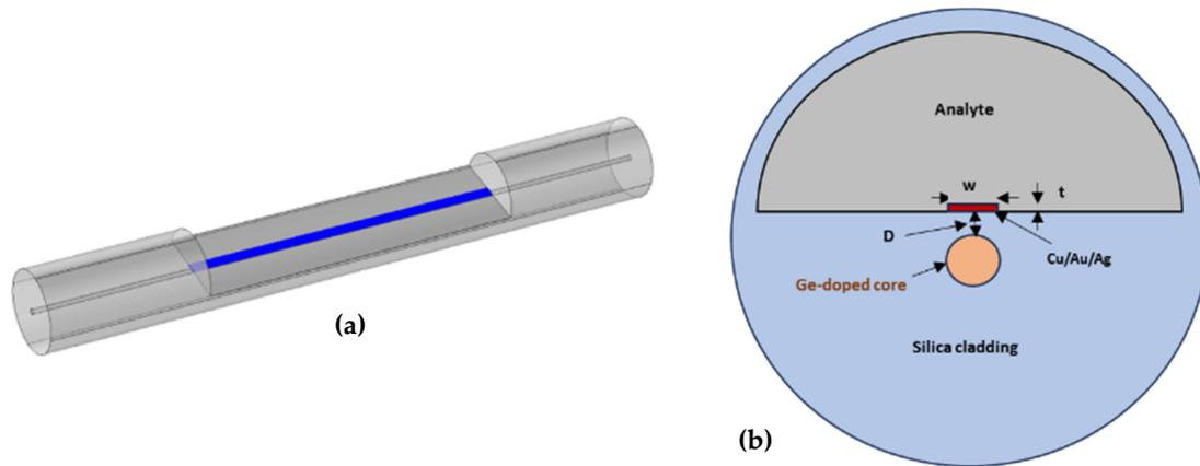
**Figure 1.** (a) 3D schematic of D-SPR sensor; (b) 2D sensor design showing the design parameters.
