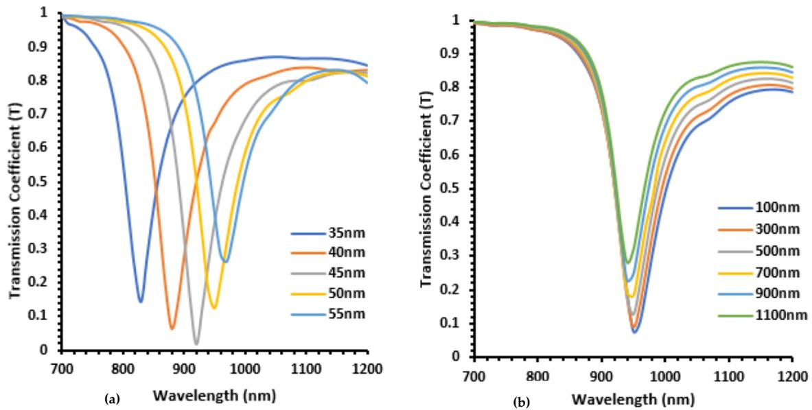
**Figure 3.** Transmission spectra for different (a) thicknesses of Ag thin film; (b) residual cladding thickness (D) of sensor design.
