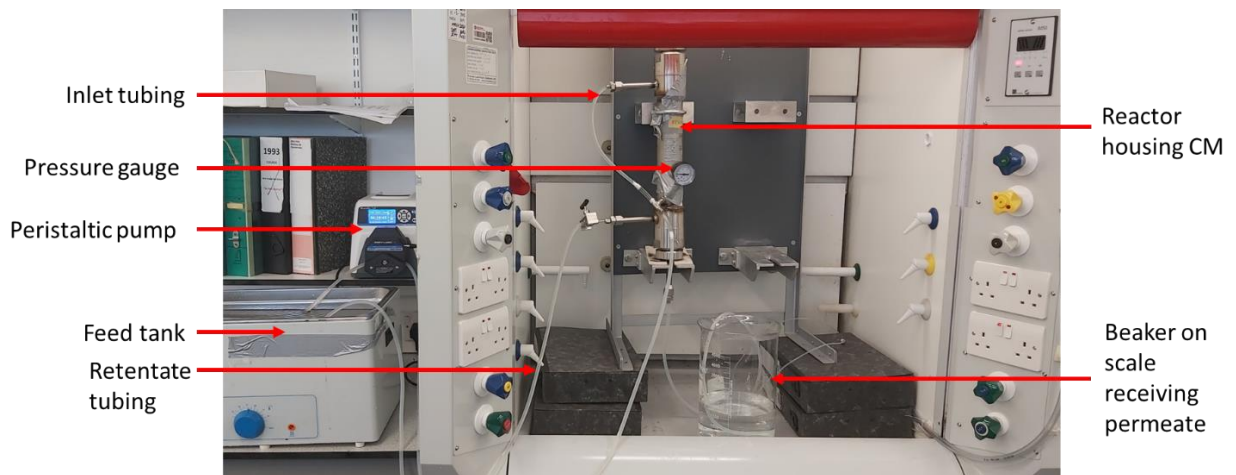
Figure 36: Rig for O/W emulsion crossflow nanofiltration.
