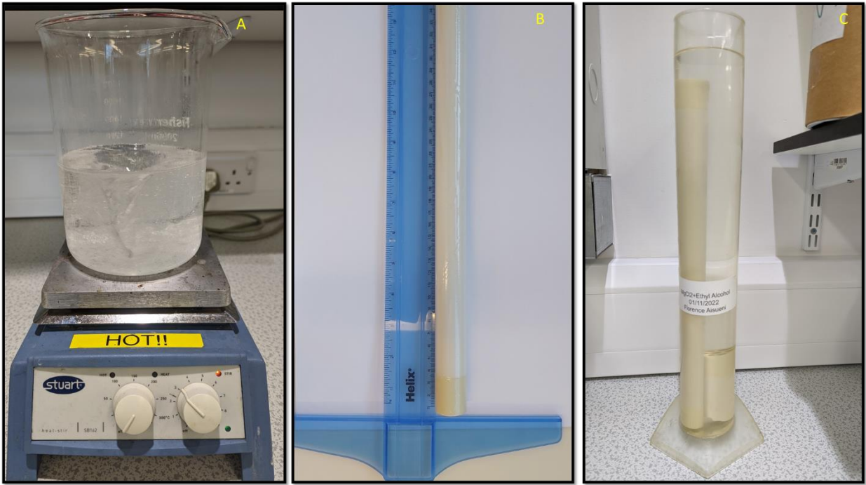
Figure 28: A-MgCl 2 solution, B-fresh support ceramic membrane, C- Ceramic membrane and witness sample in MgCl 2 solution.
