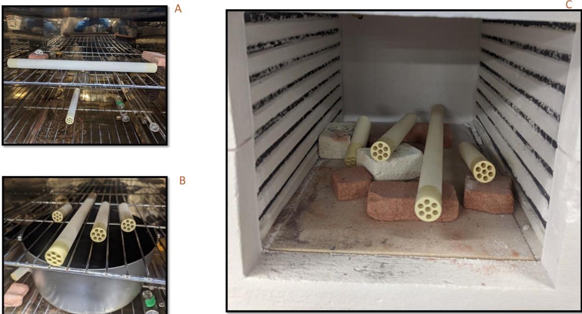
Figure 29: A-MgCl 2 solution, B-fresh support ceramic membrane, C- Ceramic membrane and witness sample in MgCl 2 solution.
