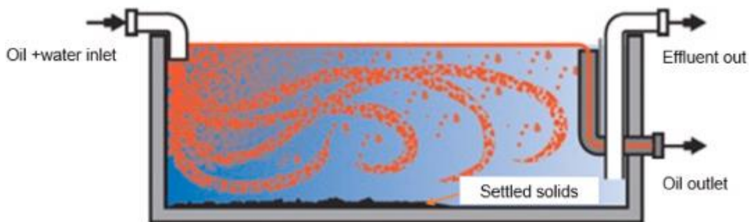
Figure 6: Schematics of API oil-water separator. (Amakiri et al. 2022).
