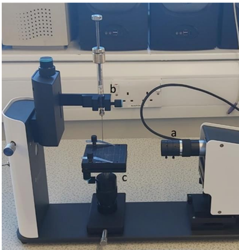
Figure 26: Image of OneAttention Theta Lite Optical Tensiometer - adapted from Biolin Scientific Manual. (a – camera area, b - syringe in syringe holder for sample liquid phase injection, c – sample stage for any solid sample placement).
