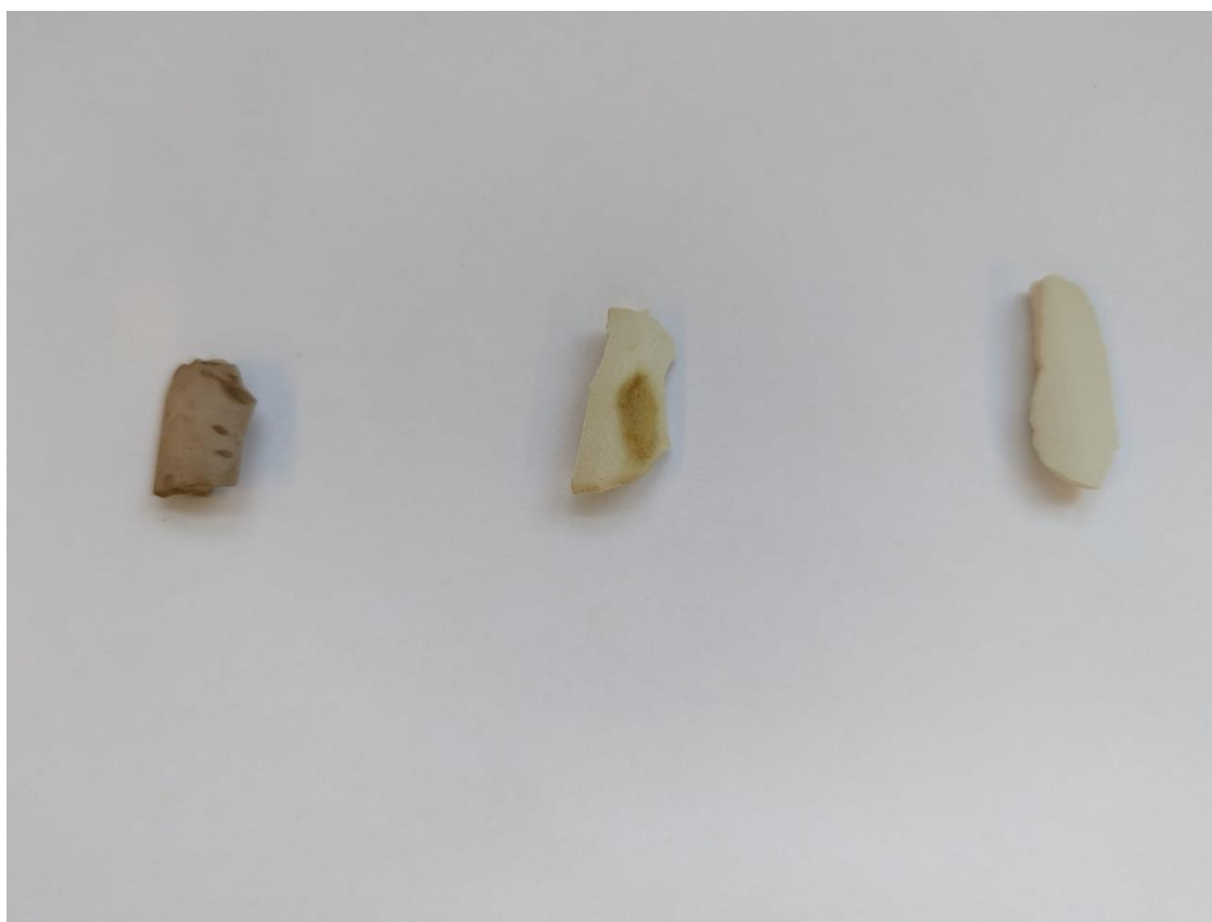
Figure 46: From left to right – MnO, CrO 2 , and MgO modified ceramic membrane witness samples.
