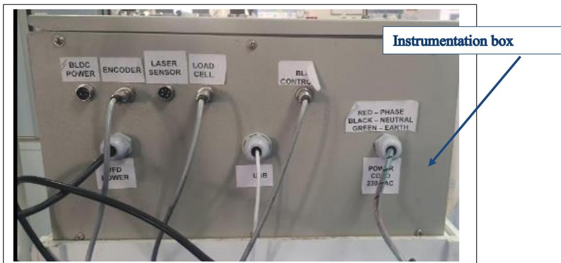
Figure 7.9: Instrumentation box and sensor connections.
