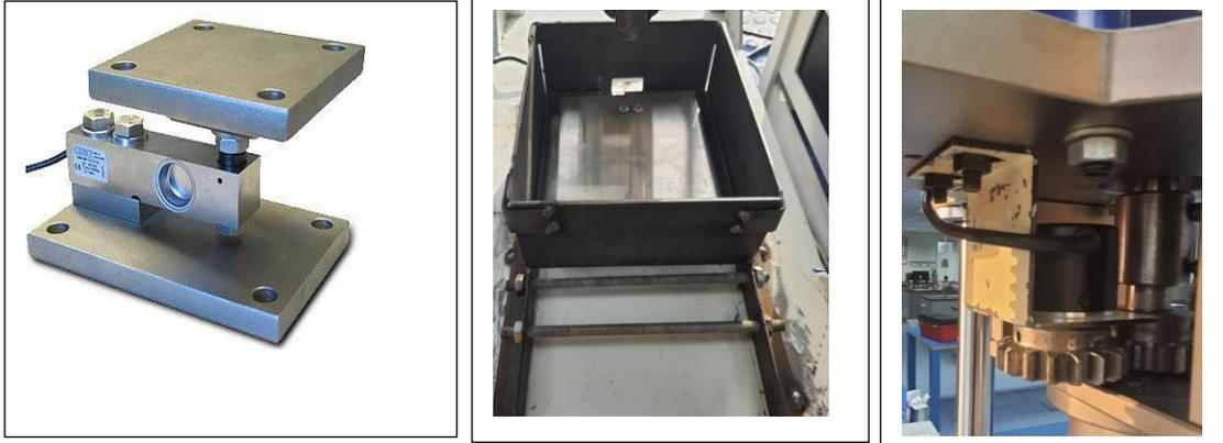
Figure 7.8: (a) Loadcell (b) Installed loadcell on core holder, (c) Position of rotary encoder.
