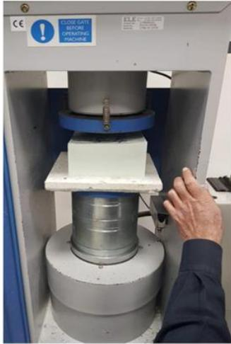
**Figure 7.2:** Experimental testing of Core UCS using ADR1500. Machine
