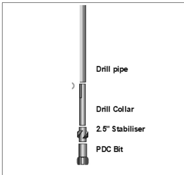
Figure 7.11 : Bottom Hole Assembly Design
