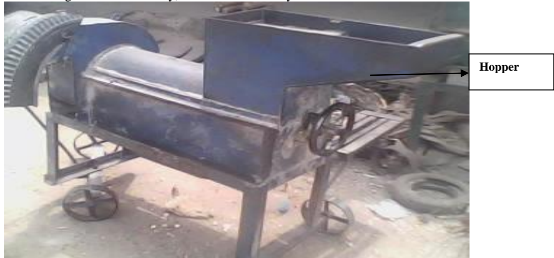
Plate 1: Locally Fabricated Maize Sheller showing the Hopper
