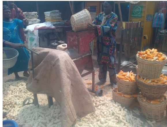
Plate 3b: Cobs Outlet Covered with Sack to Prevent Flying Over
