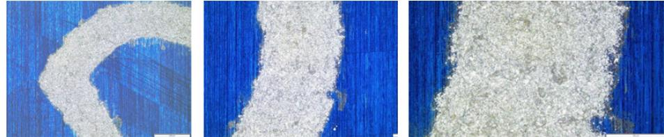
**Figure 2.** Microscopic image of printed lines on solar cells—50  $\mu\text{m}$ , 100  $\mu\text{m}$  and 200  $\mu\text{m}$ .
