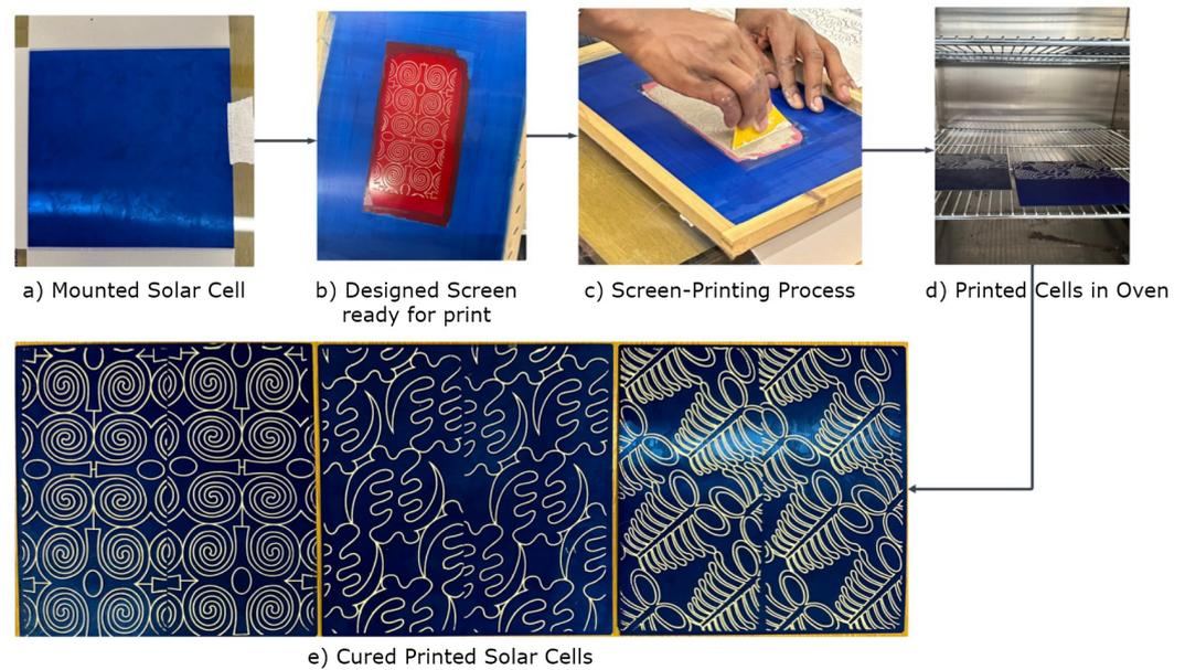
**Figure 1.** Diagrammatic illustration of the screen-printing process.
