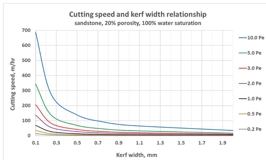
**Fig. 2.** Cutting speed and kerf width relationship (sandstone, 20 % porosity, 100 % water saturation).
