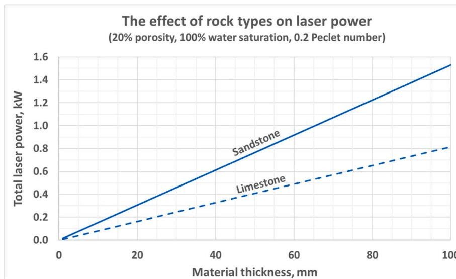
Fig. 6. The effect of rock types on laser power (20 % porosity, 100 % water saturation, 0.2 Peclet number).
