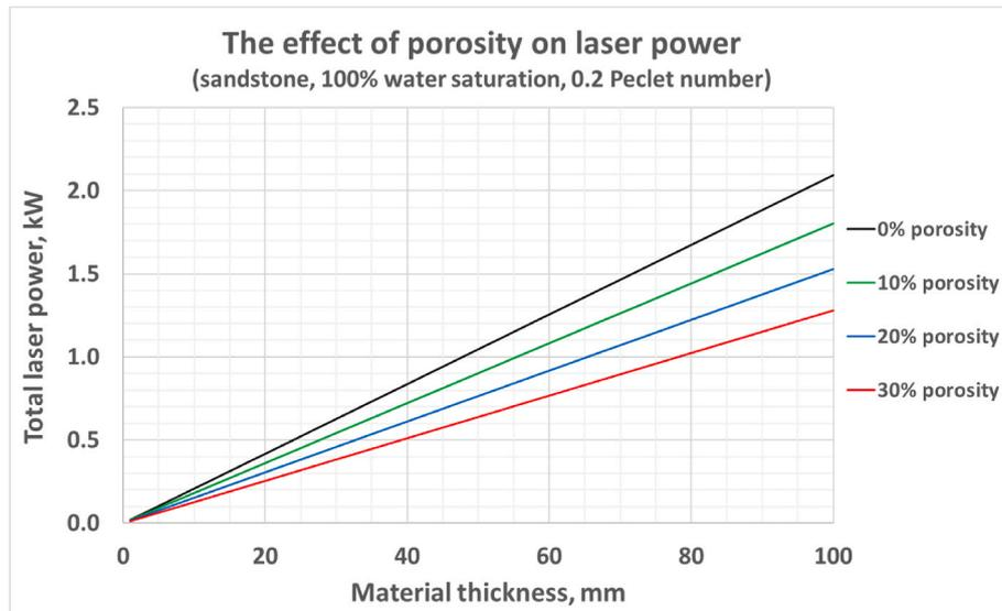
Fig. 4. The effect of porosity on laser power (sandstone, 100 % water saturation, 0.2 Peclet number).
