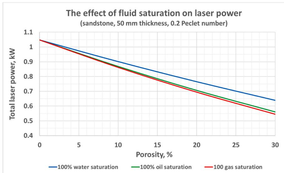
Fig. 5. The effect of fluid saturation on laser power (sandstone, 50 mm thickness, 0.2 Peclet number).
