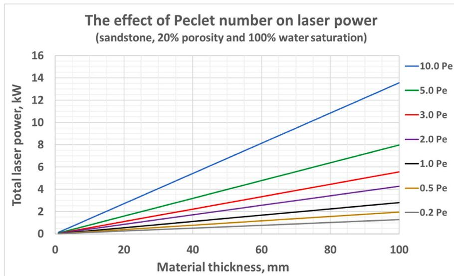
Fig. 3. The effect of Peclet number on laser power (sandstone, 20 % porosity, 100 % water saturation).
