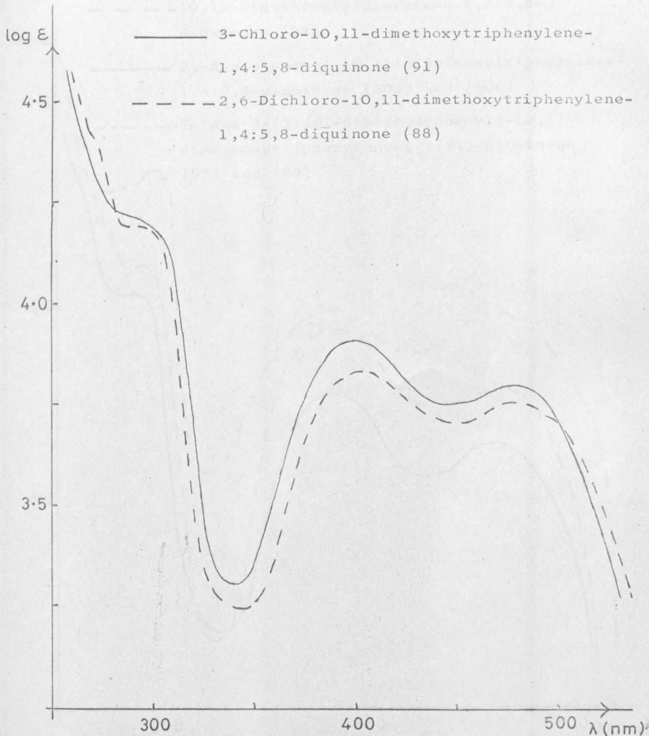
Figure 4 U.v. absorption (in  $\text{CHCl}_3$ ) of Pummerer's quinone and its methyl- and aryl-derivatives
