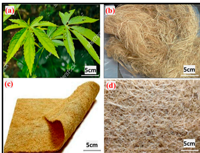
Figure 1. Pictorial image of (a) kenaf plant (b) kenaf fiber (c) needle-punched woven kenaf (d) microscopic view of nonwoven kenaf fibre.
