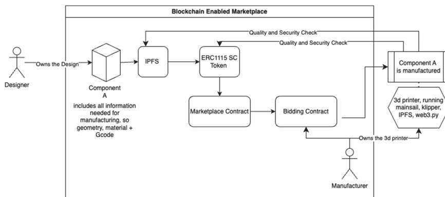
Figure 1: Printing a 3d component with the use of a smart contract and IPFS
