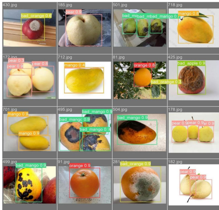
Fig. 12. Fresh and defective fruit detection results using the proposed FRYOLO network model.
