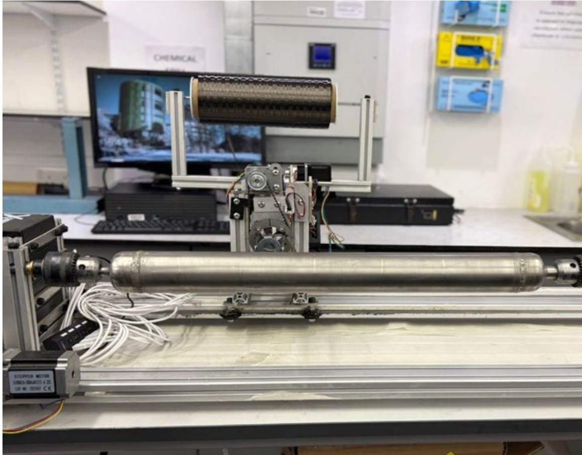
Filament Winding – Composite cylinder manufacturing
