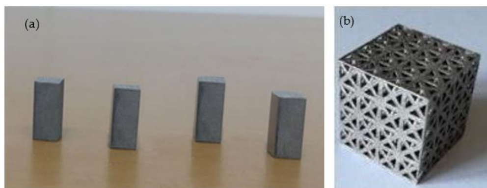
Figure 5. Ti-6Al-4V samples fabricated using LPBF: (a) LPBF coupons for compression-testing properties; (b) optimised lattice design.
