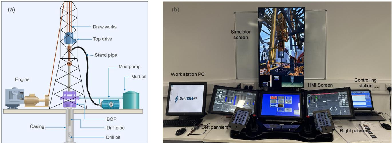
Fig. 2. OTR simulator in the experimental room. The main simulation computer is connected to a workstation PC, HMI, and an instructor laptop. The workstation PC hosts the API for different rig packages and is used to collect data from the simulator. The instructor's laptop is used to set drilling scenarios based on geological data.
