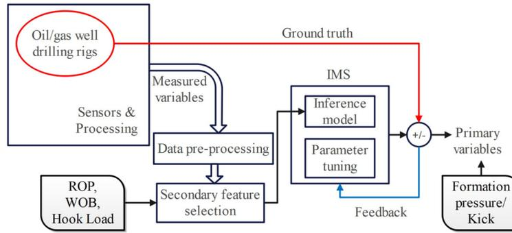
Fig. 1. Overview of the inferential measurement system (IMS) architecture for drilling rigs. The sensors and actuators are connected to the drilling rigs to measure different drilling variables. After preprocessing, the secondary variables related to the primary variable are chosen. The inference model is then used to predict the primary variable, such as formation pressure from the secondary variables. The inference model can also take feedback from the predicted data and update its parameters.
