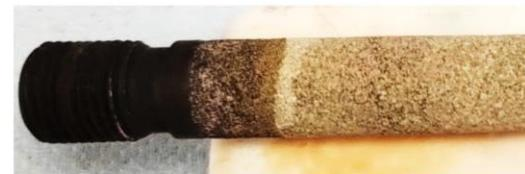
Ultrasonicated slurries, high-temperature sintering (950-1100 C)
