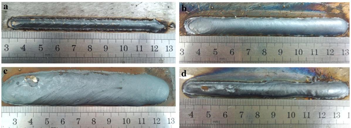
**Fig. 6.** Various forming appearances with different combinations of process parameters (a) an incomplete fusion of weld toe, (b) excellent appearance (c) overflowing, and (d) hump and scallop [97].
