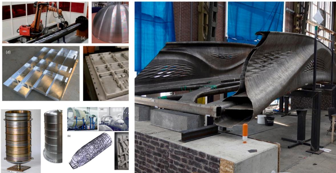
Fig. 19. Various WAAM applications.
