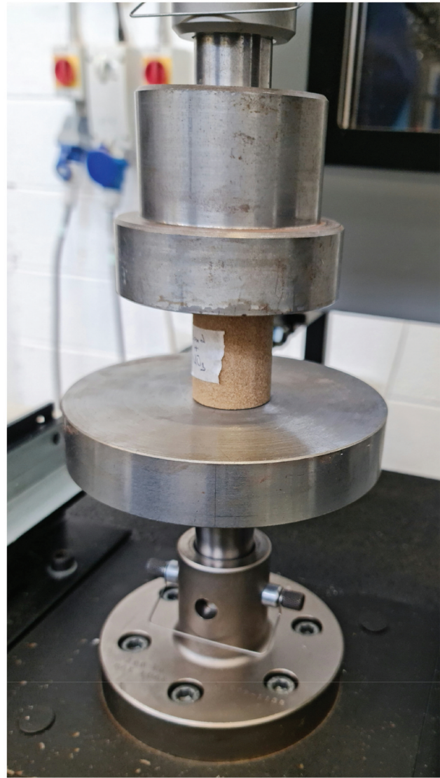
Figure 1. An image of rock sample under mechanical test using instron model 3382 machine.
