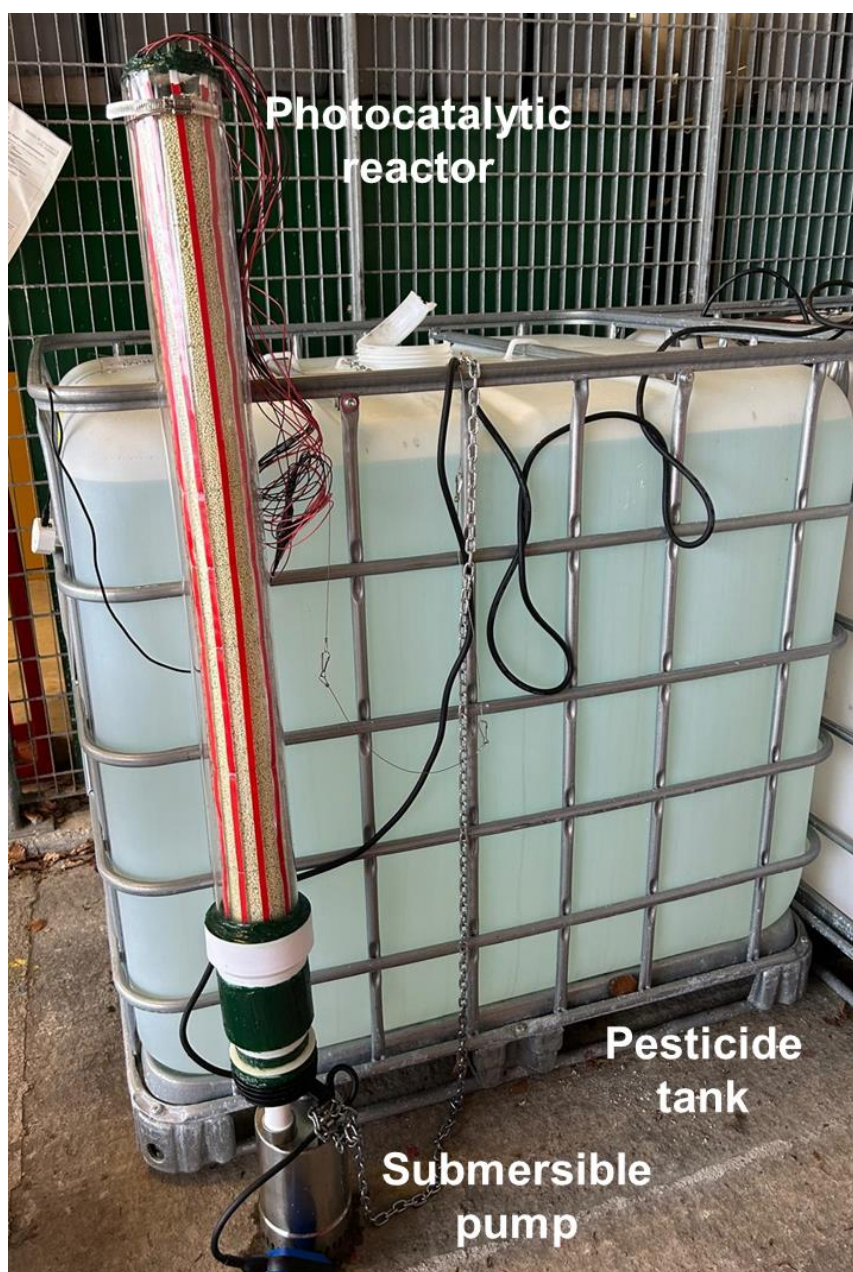
Figure 5.1: Photocatalytic reactor based on graphitic carbon nitride ( g\text{-C}_3\text{N}_4 ) coated beads and UV-A LEDs (365 nm) connected to submersible water pump and tank containing diuron experimental solution.
