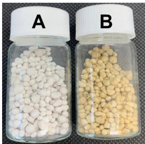
Figure 3.5: A) Titanium dioxide ( \text{TiO}_2 ) and graphitic carbon nitride ( \text{g-C}_3\text{N}_4 ) coated glass beads to be used as catalysts during heterogenous photocatalysis.
