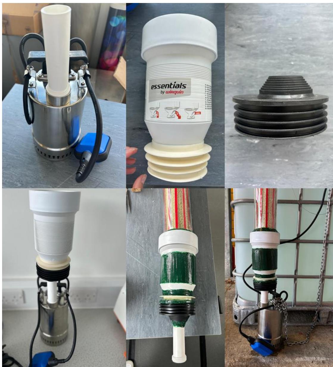
Figure 5.11: Submersible water pump connected to the photocatalytic reactor for the removal of diuron at large-scale in a 1000 L tank.
