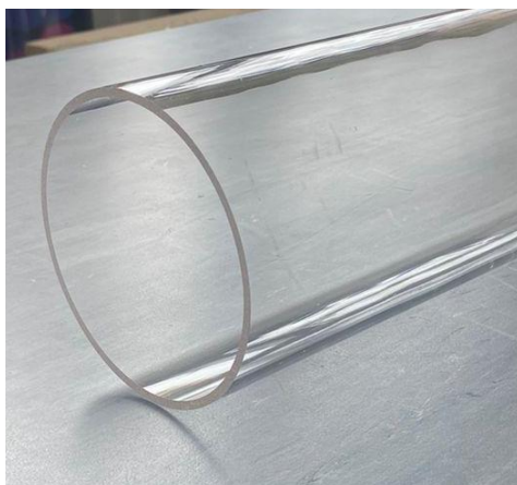
Figure 5.4: Acrylic tube evaluated as material during construction of photocatalytic reactor prototype.
