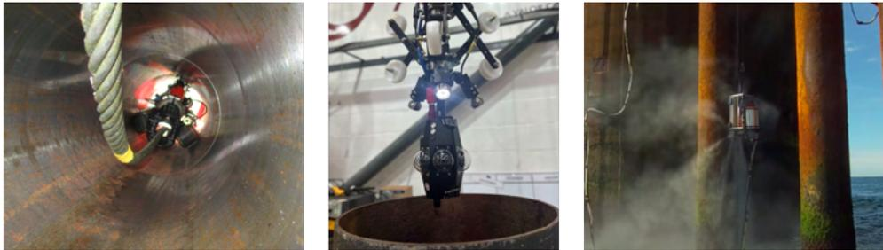
Figure 3.3: Inspection Vehicles for Visual Inspection
