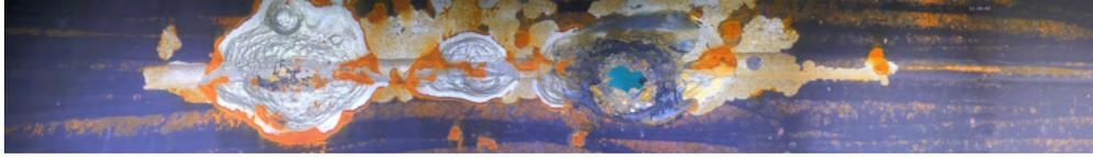
Figure 2.3: Example of a 180° internal panoramic view of a component circumferential weld with defects.
