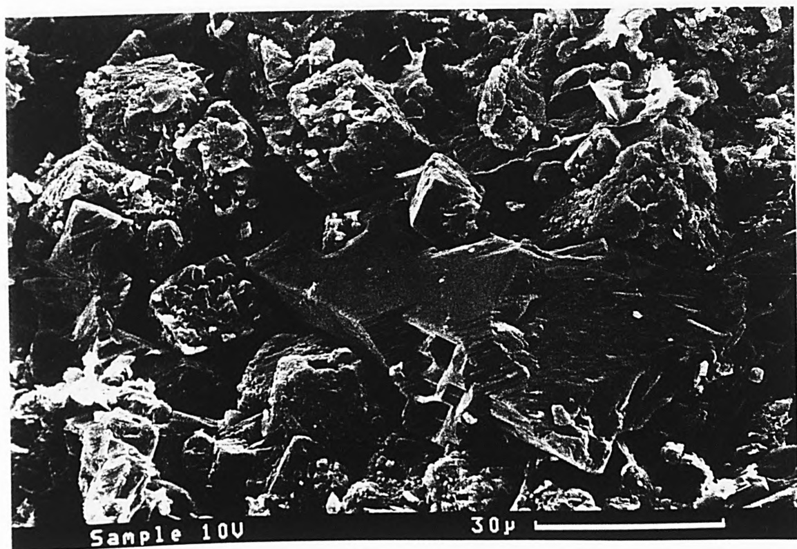
Fig. 6.6 Coarse stepped crystals are anhydrite which may formed replacively. Micropores and macropores are presence and it reflect heterogeneity of this sample. Large pores may be related to dissolution-precipitation process. (sample 2; Zone C).
