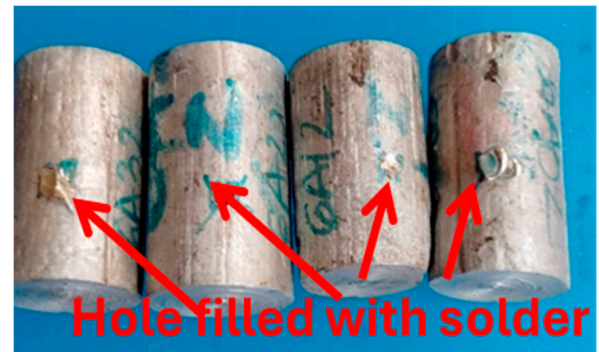
(b) Solder-filling artificial crack
