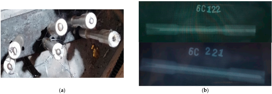
Figure 5. (a) Solder-filled tensile specimens and (b) Radiography of the solder-filled samples.
