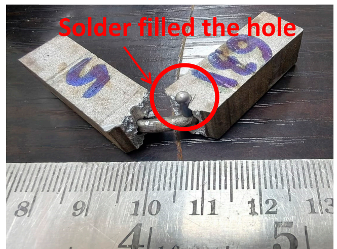
(f) Impact specimen Self-healed
