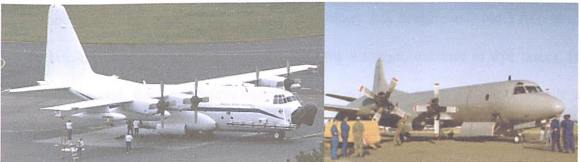
Figure 2.10: Photograph of a C-130 “Hercules”(left) and a P-3B “Orion” (right) used to house the Airborne Oceanographic Lidar
