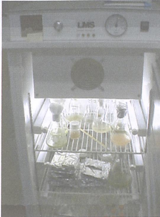
Figure 4.4 : Photograph of the cooled incubator used for growing phytoplankton
