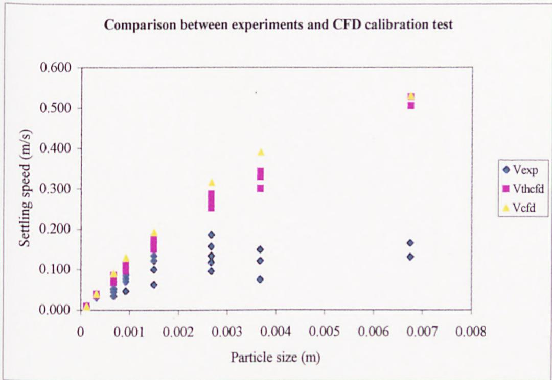
**Figure 5.6: Comparison between experiments and CFD calibration test.**
