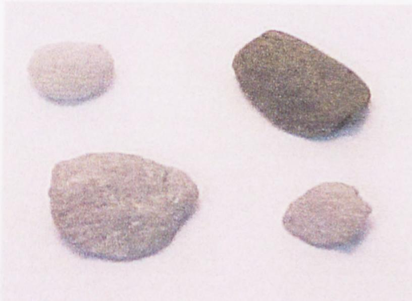
Figure 3.8: Angular-round drill-cuttings.
