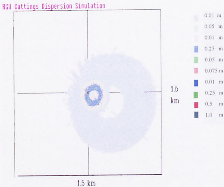
**Figure 1.3: Example of a 2D mapping of thickness profiles (in meters) from a dispersion model (Carles and Bryden 1999).**
