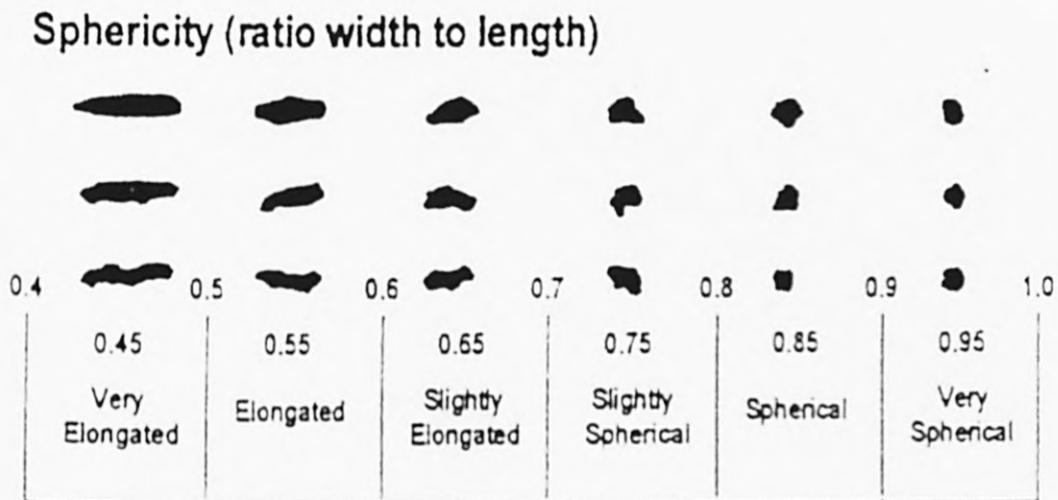
Figure 3.6 Chart for particles shape from Geoservices (1994).
