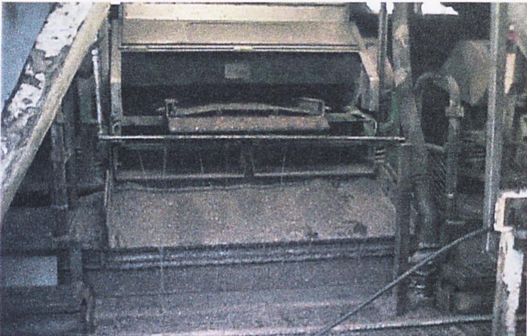
**Figure 2.6: Shale shakers separating mud and cuttings.**
