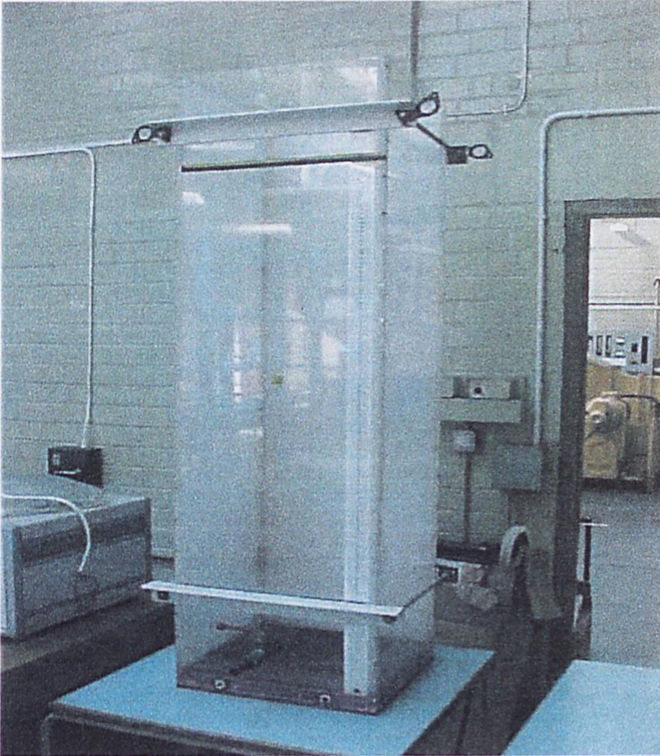
**Figure 3.15: A picture of the water tank used for the settling experiments.**
