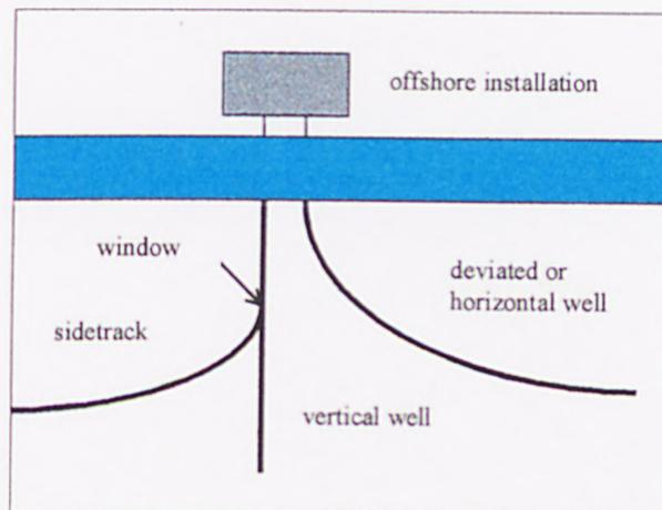
**Figure 2.4: The different features of a well.**
