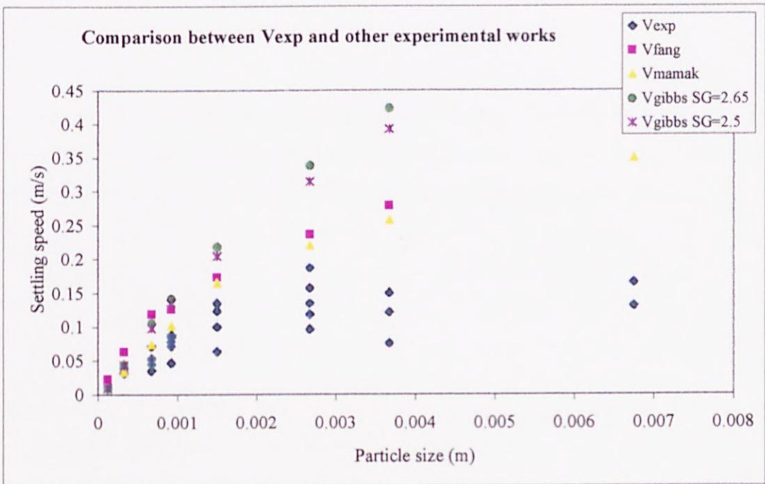
Figure 4.4: Comparison between the experimental values and other works.
