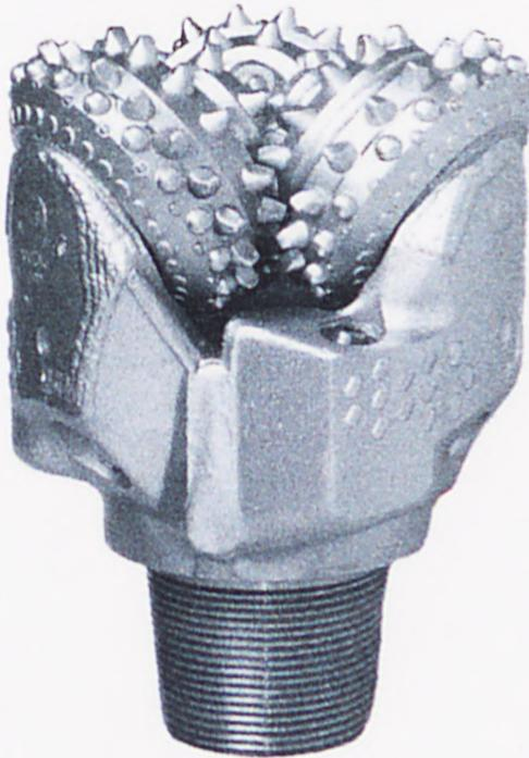
Figure 2.9: An example of an insert bits (Courtesy of Baker Hughes).
