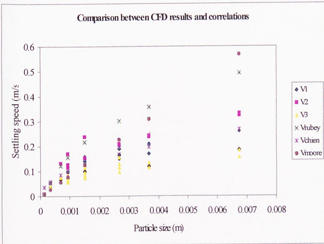
Figure 5.11: Comparison between CFD results and correlations.
