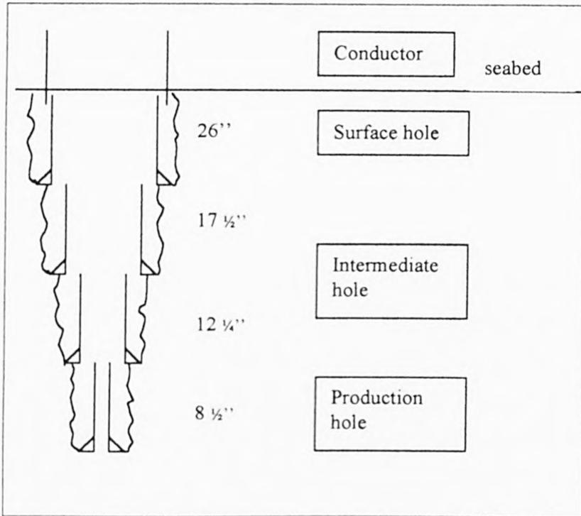
**Figure 2.3: An example of the different well sections.**
