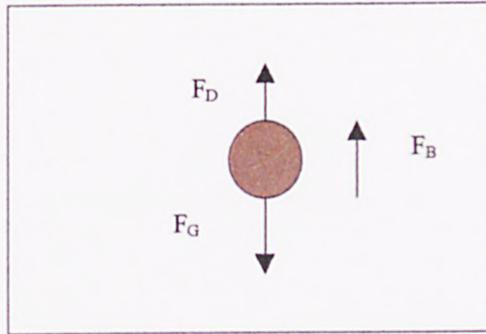
**Figure 4.1: The forces applied to a particle (Naik 1996).**
