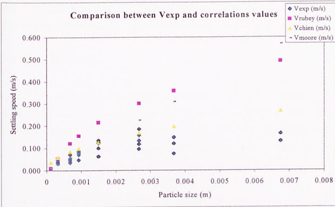
**Figure 4.5: Comparison between the experimental values and correlations.**
