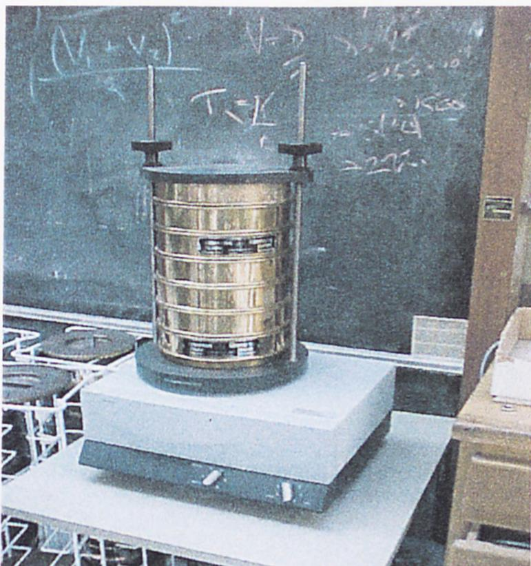
**Figure 3.4: The stack of sieves on the analytical shaker.**
