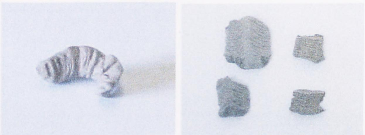
**Figure 2.11: Cuttings drilled with PDC bits.**
