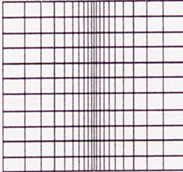
**Figure 5.3: The logarithmic mesh of the inlet and outlet of the modelled tank.**
