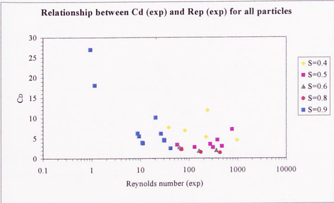
**Figure 4.7: Experimental values for Reynolds number and drag coefficient of particles.**
