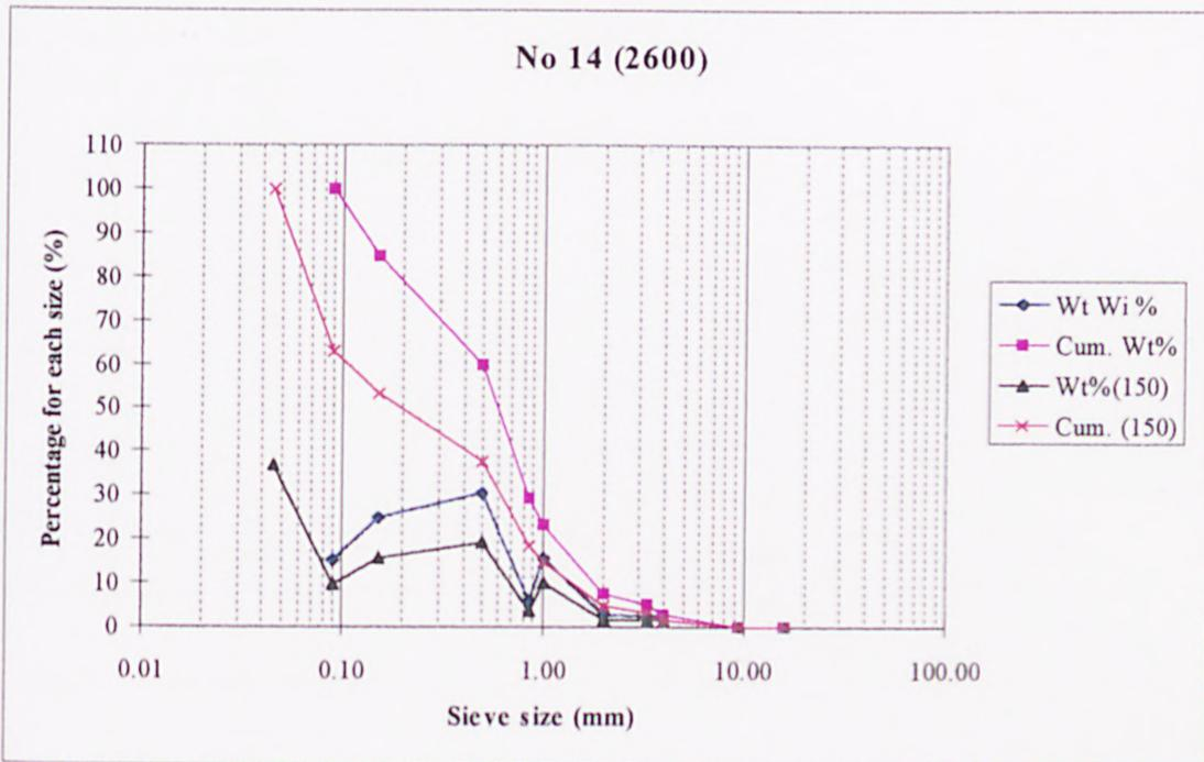
**Figure 3.13: Two examples of graphs from sieving data.**
