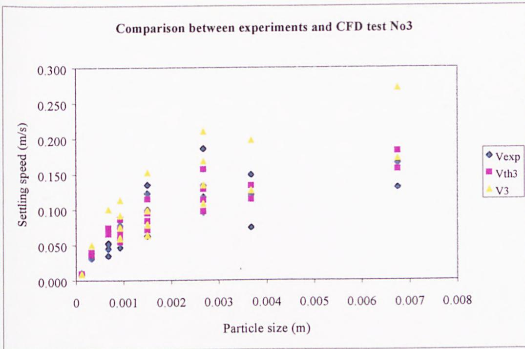
**Figure 5.9: Comparison between  $v_3$ ,  $v_{th3}$  and  $v_{exp}$ .**
