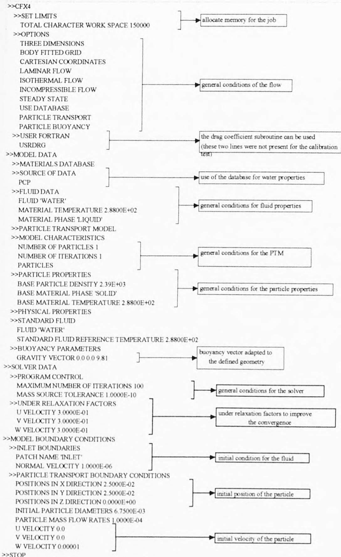
Figure 5.4: The command file used for the CFD tests.
