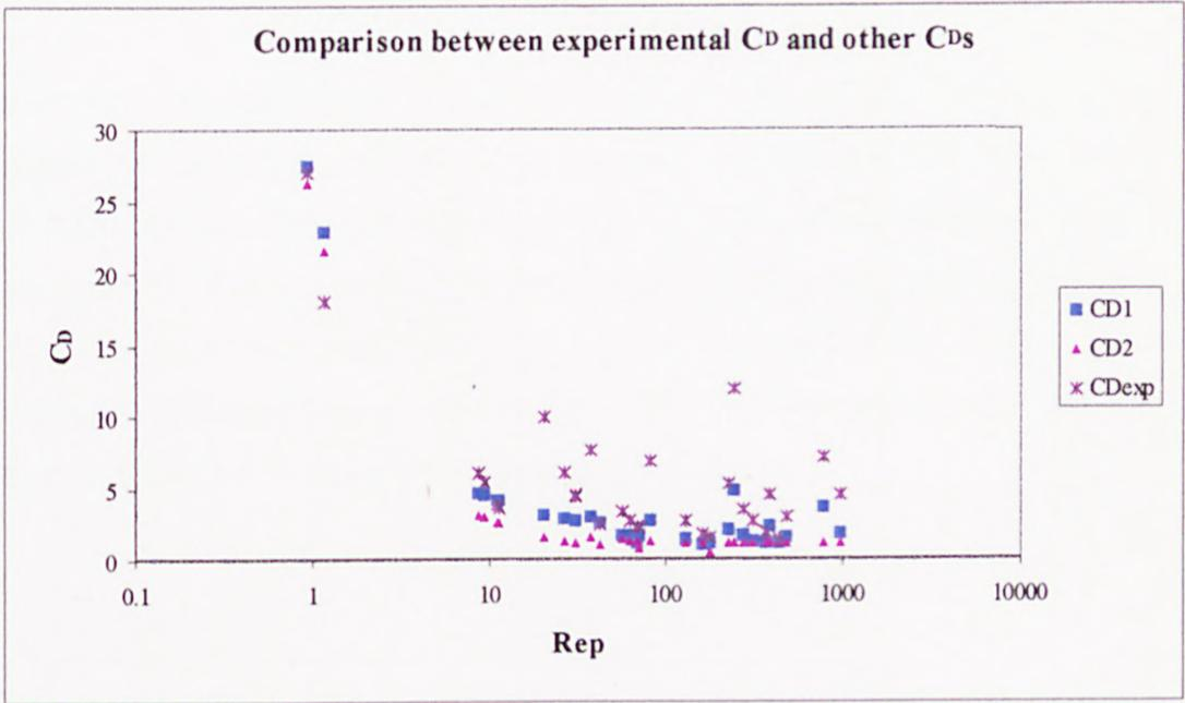
**Figure 4.8: Comparison between the experimental values for  $C_D$  and  $Re_p$  and the correlations values.**
