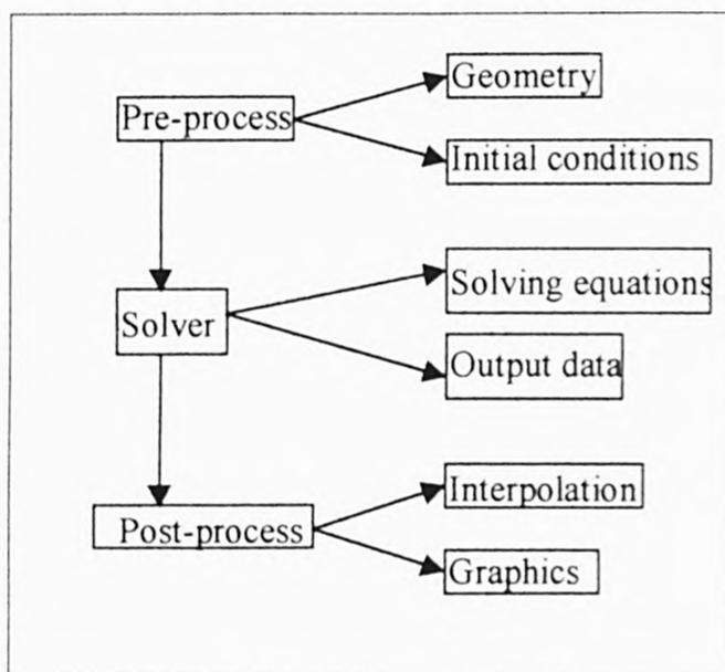
**Figure 5.1: The structure of a CFD package.**
