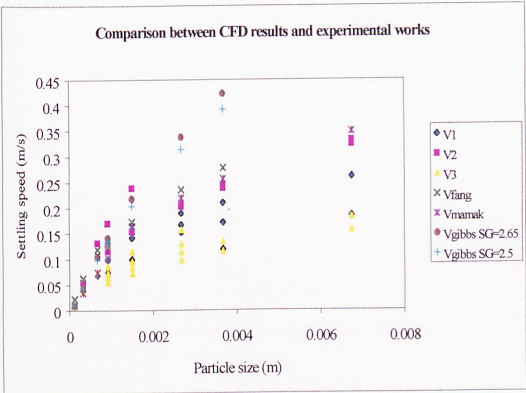
Figure 5.10: Comparison between CFD results and experimental works.
