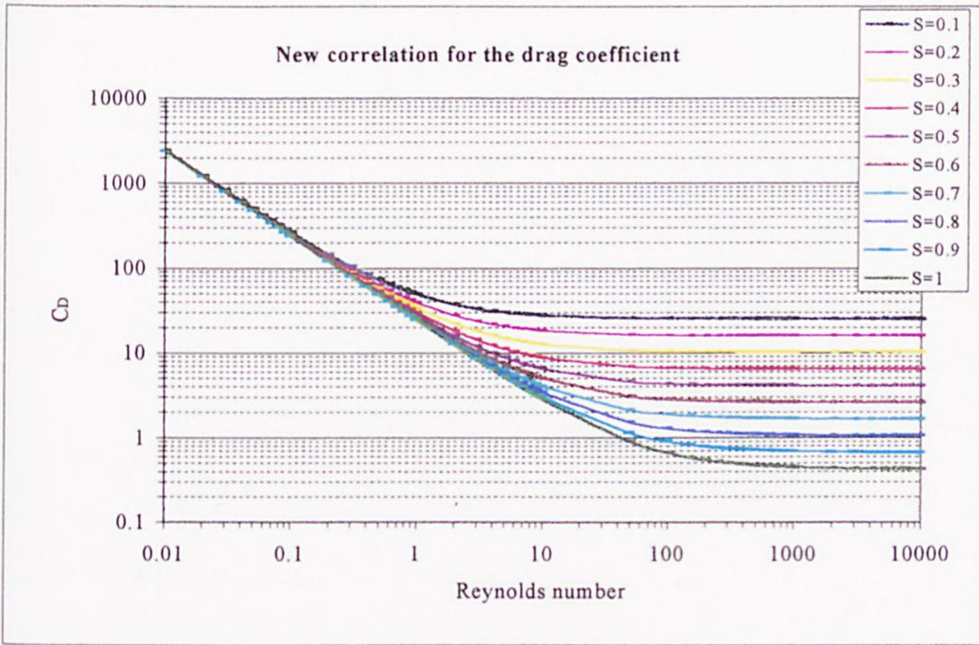
**Figure 4.9: The new correlation for the drag coefficient.**
