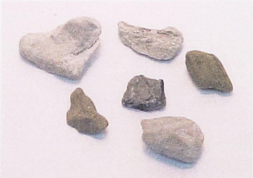
**Figure 3.10: Angular-flat drill-cuttings.**
