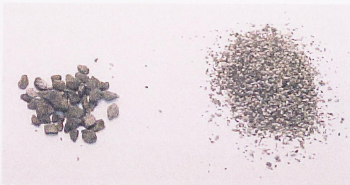
**Figure 3.12: Small drill-cuttings assumed to be very round.**
