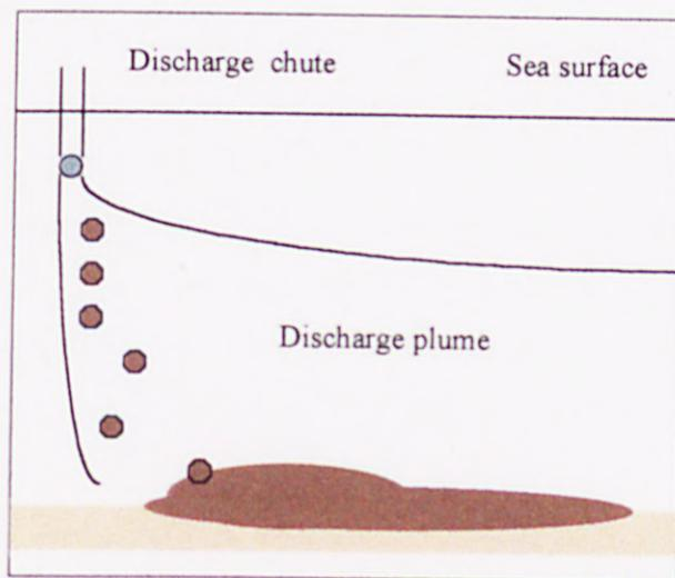
**Figure 1.2: The transport of discharged material into the sea.**
