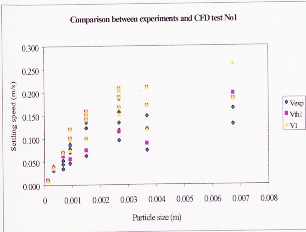
**Figure 5.7: Comparison between  $v_l$ ,  $v_{th1}$  and  $v_{exp}$ .**
