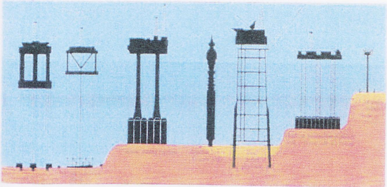
**Figure 2.1: The different types of rigs (UKOOA 1997).**
