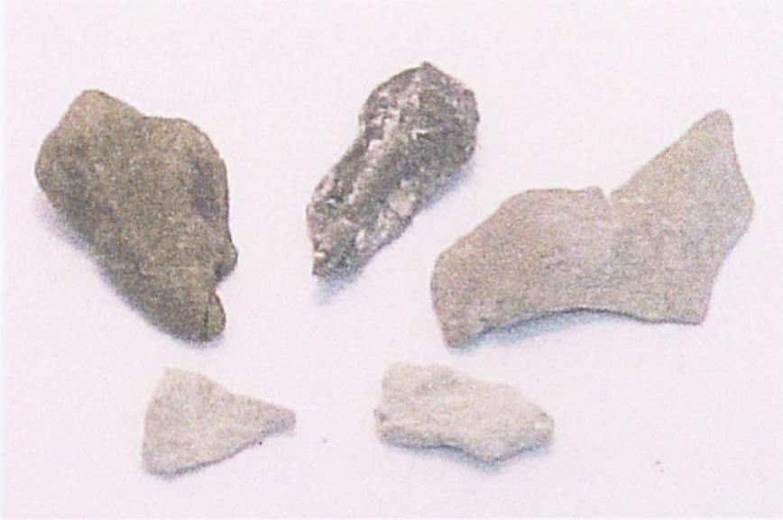
**Figure 3.9: Angular drill-cuttings.**
