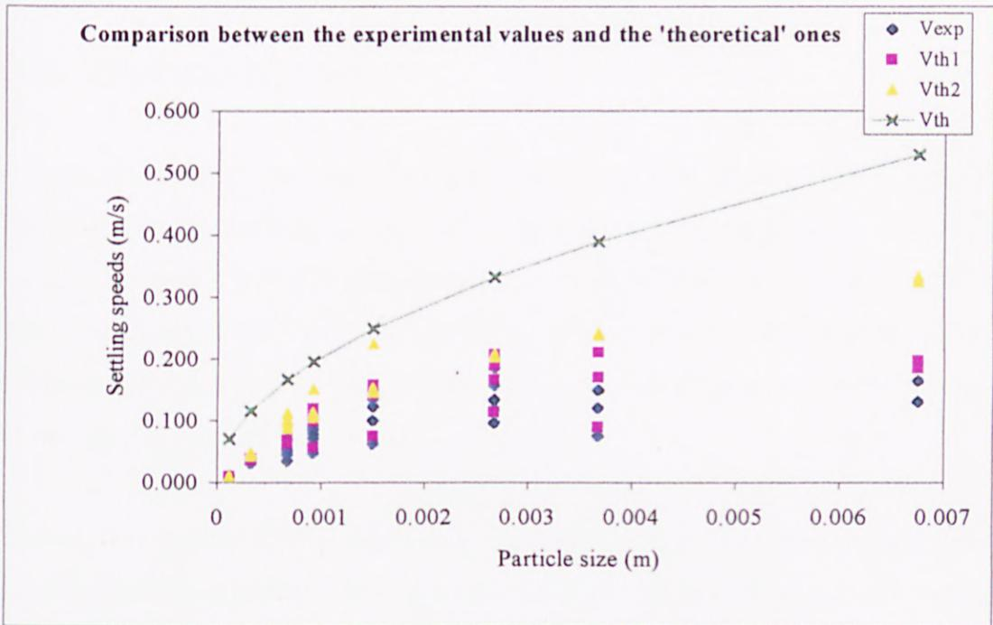
**Figure 4.3: Comparison between experimental settling speeds and theoretical values.**
