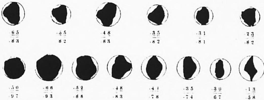
Figure 3.5 Chart for particles shape from Wadell (1932).
