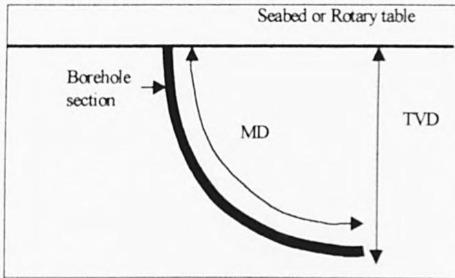
**Figure 3.2: The difference between the TVD and the MD.**
