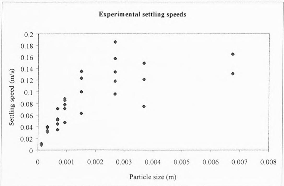
**Figure 3.17: Experimental settling speeds values.**
