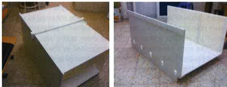
Figure 1. the scale model (left) The openings in the walls to place the probes of the Light-meter (right)
