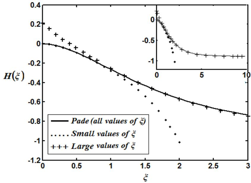
**Fig. 2(c).** Comparison of our axial velocity component  $H(\xi)$  (Padé approximation Eq. (D5)) versus the dimensionless distance  $\xi$  with small (Eq. (3)) and long solution (Eq. (9)).
