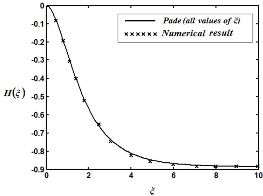
**Fig. 1(c).** Dimensionless axial velocity component  $H(\xi)$  versus the dimensionless distance profile. The key to the graph: solid line represents Eq. (D5) and the dotted line represents the numerical [3].
