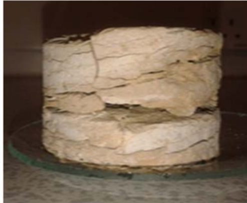
Figure 4: Damaged limestone due to treatment with ATMP.
