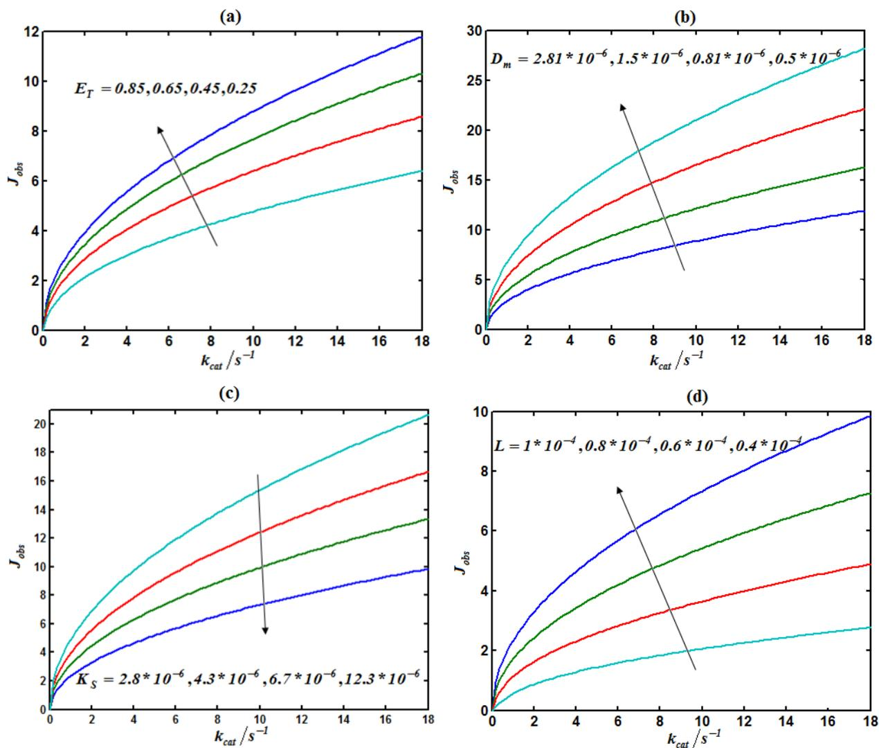
**Fig. S3.** Plot of current density versus turnover rate of GOx  $k_{cat}$  for various values of  $E_T$ ,  $d_m$ ,  $K_S$ , and  $l$ . The parameters employed are given in Table 4.
