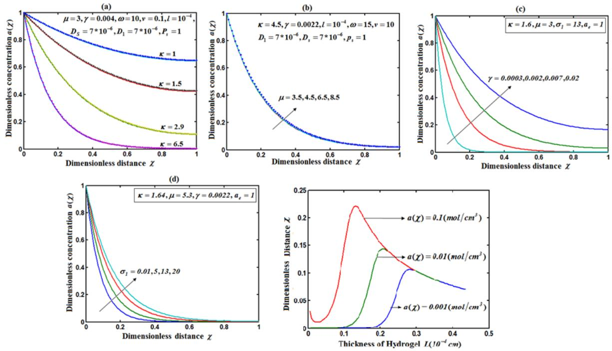
Fig 2. Comparison of dimensionless concentrations of mediator with numerical results for various values of parameter such as  $\kappa$ ,  $\mu$ ,  $\gamma$  and  $\sigma_1$ . Solid line represent Eq. (5) and dotted line represent the numerical result. Unit of all symbols are given in the nomenclature. Fig. 2e is the distance-thickness profile.
