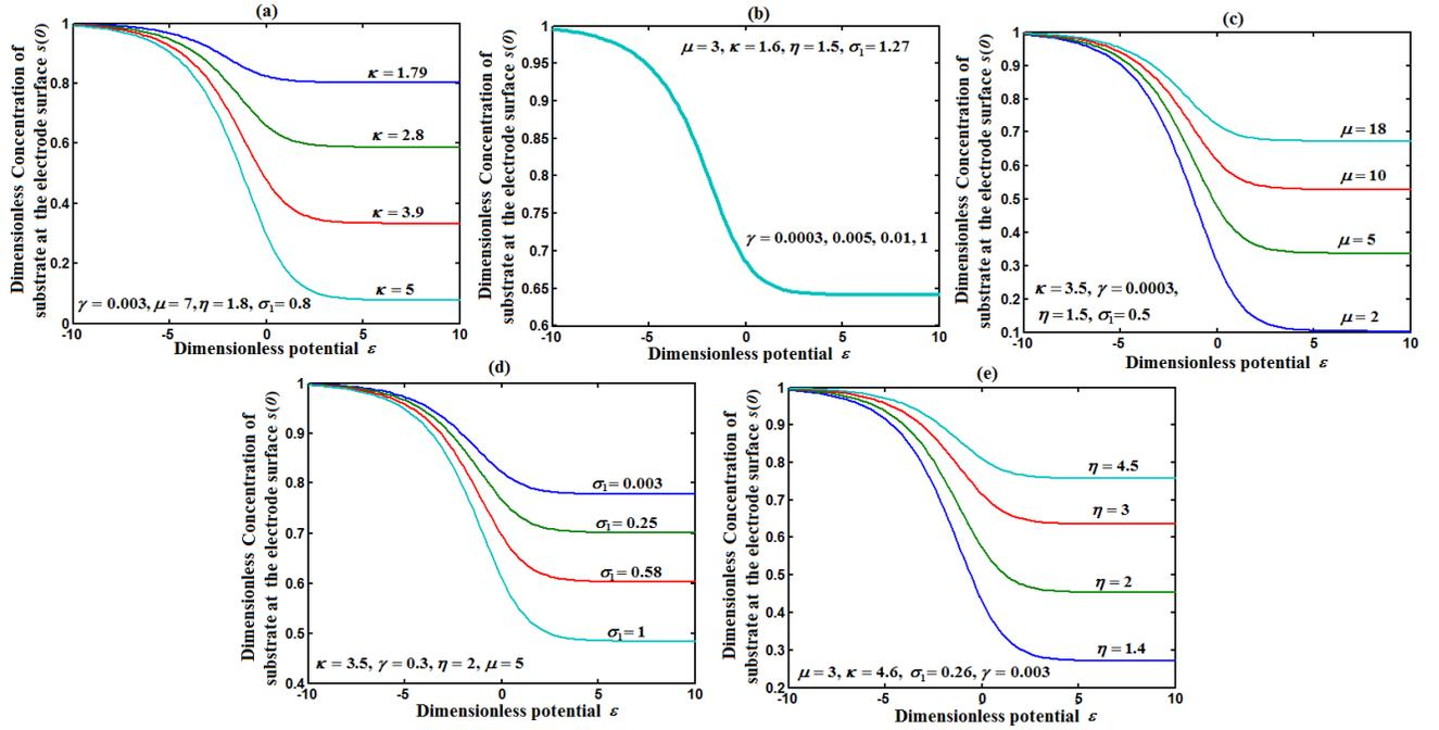
**Fig.4.** Dependence of the dimensionless concentration of substrate at electrode surface versus the potential estimated using the Eq.(10) under different values of parameters: (a)  $\kappa$ , (b)  $\gamma$ , (c)  $\mu$  (d)  $\sigma$  (e)  $\eta$
