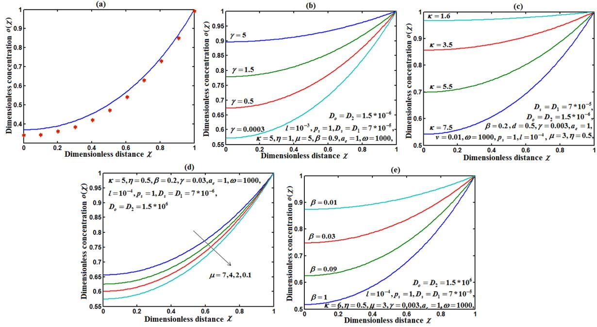
**Fig. 5.** Plot of dimensionless concentration of oxygen versus dimensionless distance from the electrode interface for various kinetic parameters using the Eq.(7). The analytical result is compared with numerical result in Fig. 5a. The values of the parameters used and unit of all symbols are given in Table 1f and nomenclature.
