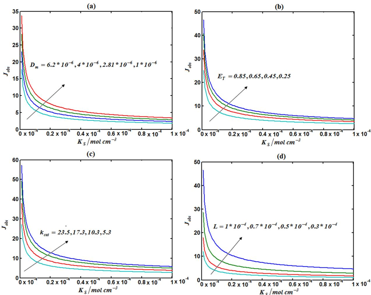
**Fig. S4.** The plot of variation of the current density with Michaelis constant for substrate  $K_S$  for various values of  $E_T$ ,  $d_m$ ,  $k_{cat}$  and  $l$ . The parameters employed are given in Table 3.
