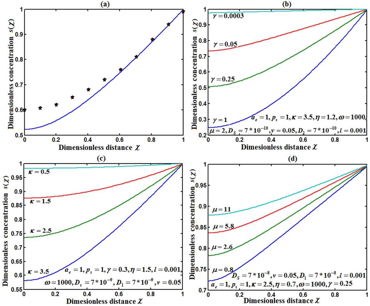
**Fig. 3.** Plot of dimensionless concentrations of substrate versus normalized distance from the electrode interface for various values of parameters such as  $\gamma, \kappa$  and  $\mu$  using the Eq.(6). our analytical result is compared with numerical results in Fig. 3a for the experimental values of parameters which are given in Table 1f. Unit of all symbols are given in the nomenclature.
