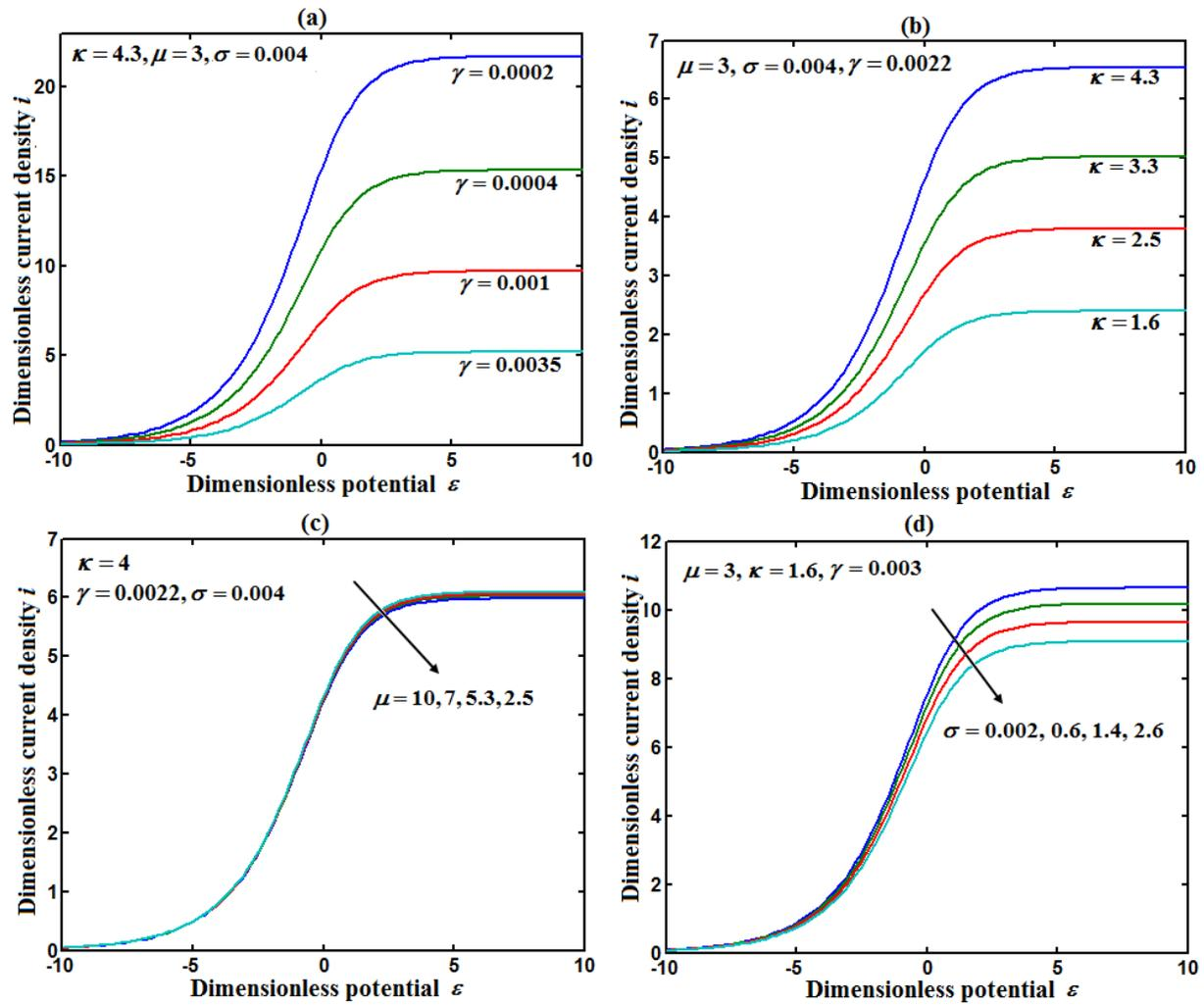
**Fig.7.** Variation of the steady state current on potential estimated using the Eq.(12) for different values of parameters:  $\gamma, \kappa, \mu$  and  $\sigma$ .
