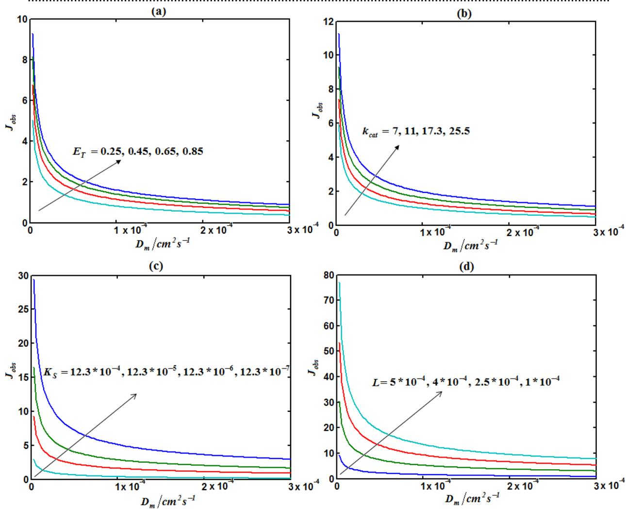
**Fig. S1.** Plot of the variation of the current density with diffusion coefficient of the mediator  $d_m$  for various values of  $E_T$ ,  $k_{cat}$ ,  $K_S$  and  $L$ . The parameters employed are given in Table 1.
