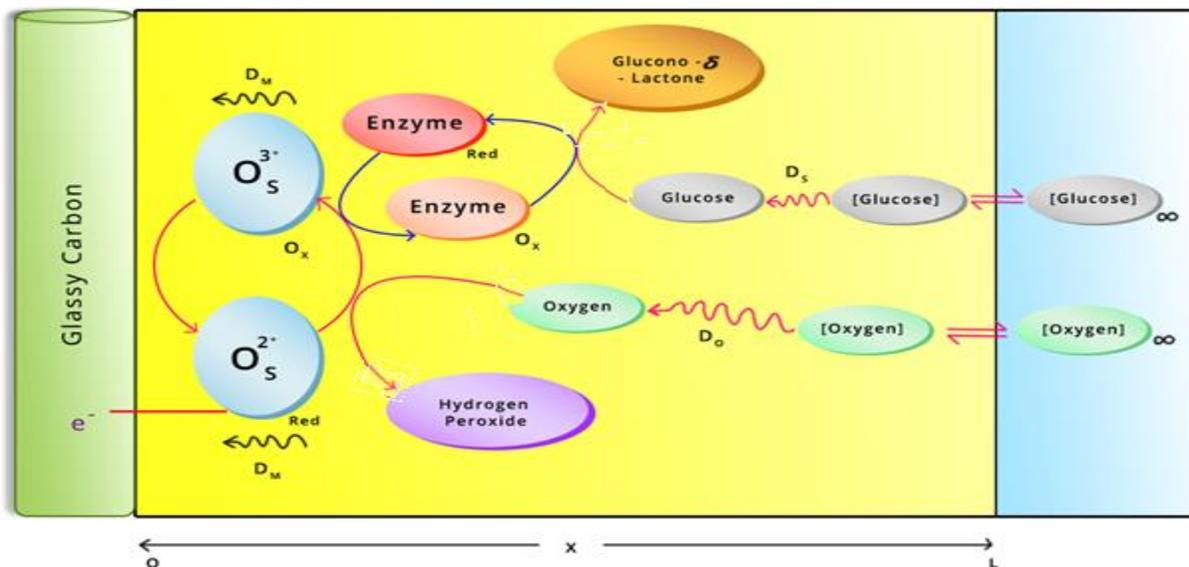
Fig 1. Systematic diagram of osmium-based redox polymer mediator glucose oxidized electrodes
