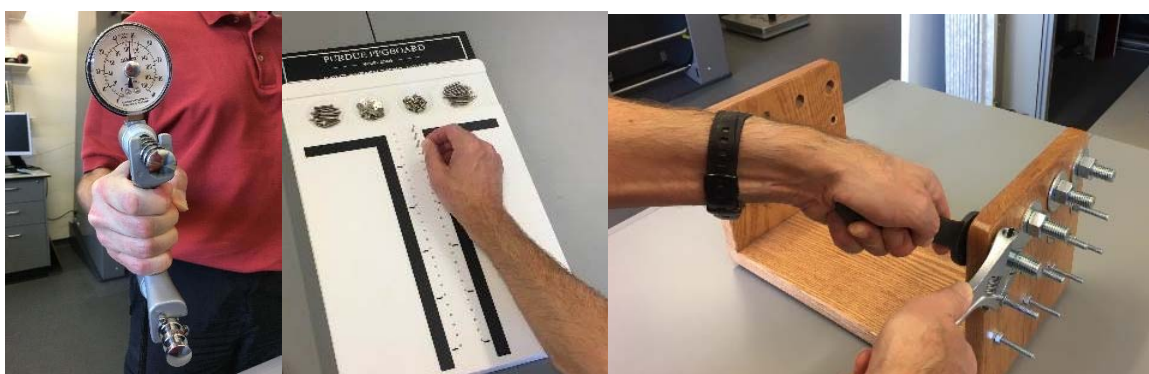
Figure 1. Left: Grip strength dynamometer; Centre: Purdue Pegboard; Right: hand tool dexterity
