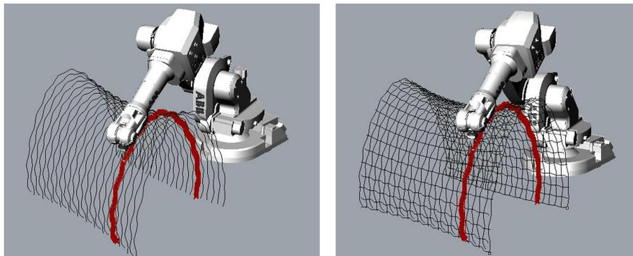
Figure 7. The sequence of weaving the vault structure though robotic simulation.
