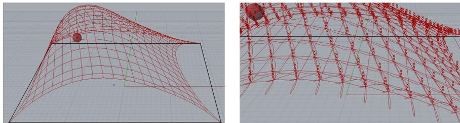
Figure 3. Grid generation and wefts control.
