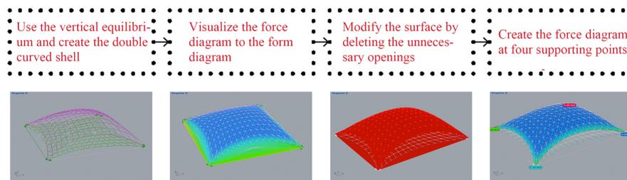
Figure 4. A double curved shell structure designed by Rhino Vault.
