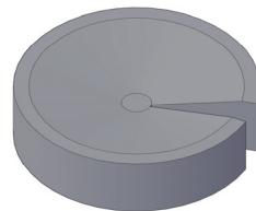
Figure 6: Joint cutout to allow members insertion
