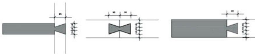
*Figure 3: Dovetail geometry according to carpentry thumb rules*
