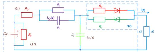
Fig. 4. The splice equivalent circuit model
