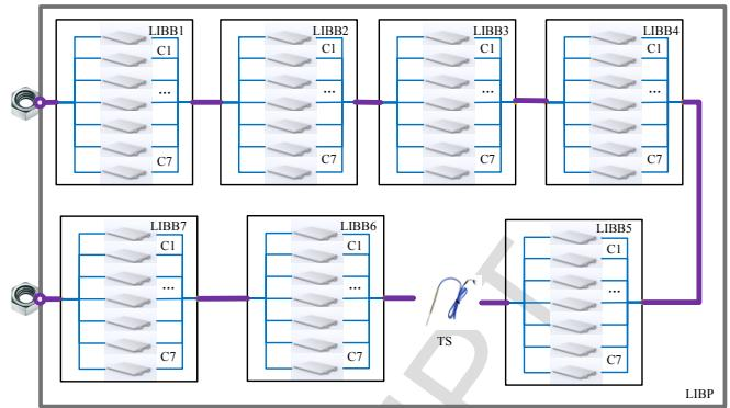
Fig. 1. The representative structure of the lithium-ion battery packs
