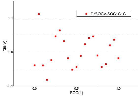
Fig. 14. OCV-SOC curve fitting error results
