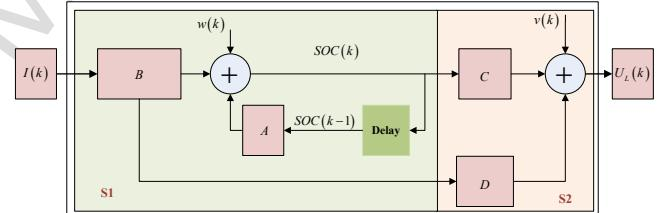
Fig. 5. The SOC estimation model framework
