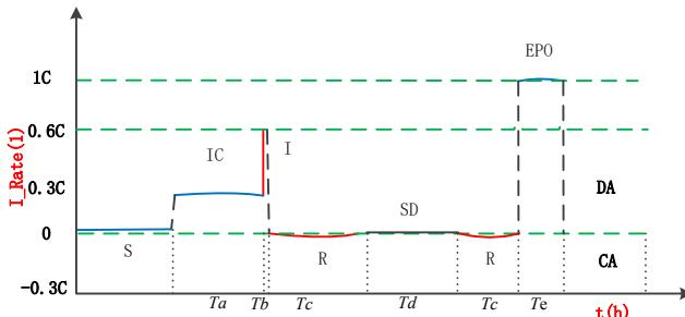
Fig. 3. The working process of aerial battery pack
