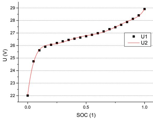
Fig. 13. OCV-SOC curve fitting effect analysis
