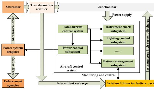
Fig. 2. The energy system structure of the aerial battery pack
