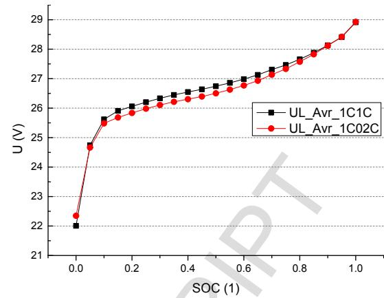
Fig. 11. The OCV-SOC relationship comparison
