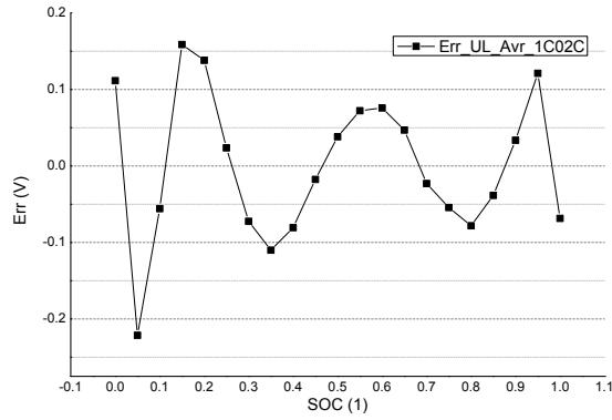
Fig. 10. OCV-SOC curve fitting error results
