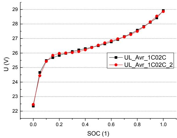
Fig. 9. OCV-SOC curve fitting effect analysis
