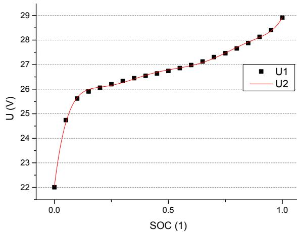
Fig. 13. OCV-SOC curve fitting effect analysis
