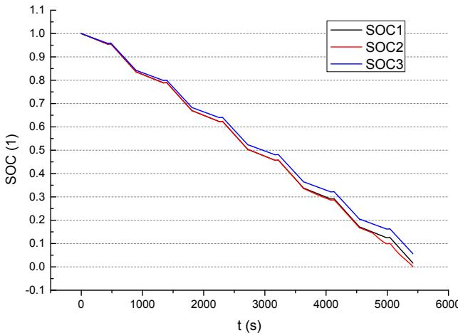
Fig. 23. Equilibrium state correction effect on the SOC estimation
