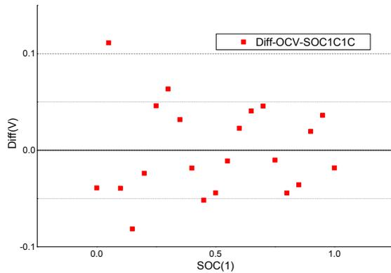
Fig. 14. OCV-SOC curve fitting error results
