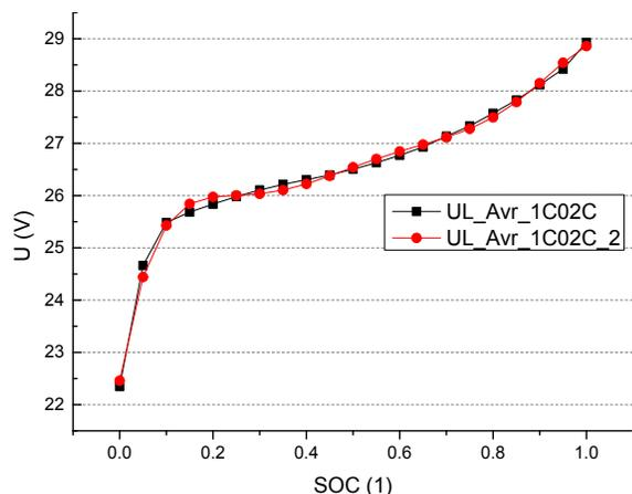
Fig. 9. OCV-SOC curve fitting effect analysis
