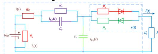
Fig. 4. The splice equivalent circuit model
