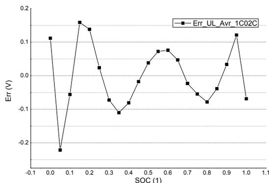
Fig. 10. OCV-SOC curve fitting error results
