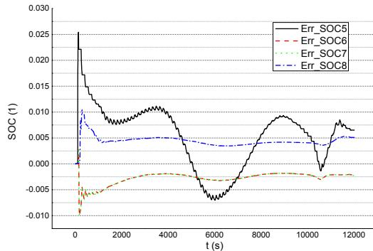
Fig. 19. SOC estimation error under different working conditions
