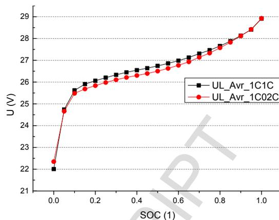
Fig. 11. The OCV-SOC relationship comparison
