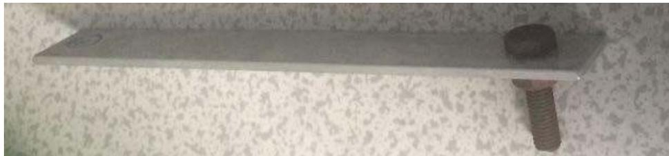
Fig. 2: Aluminium sample with steel bolt and nut
