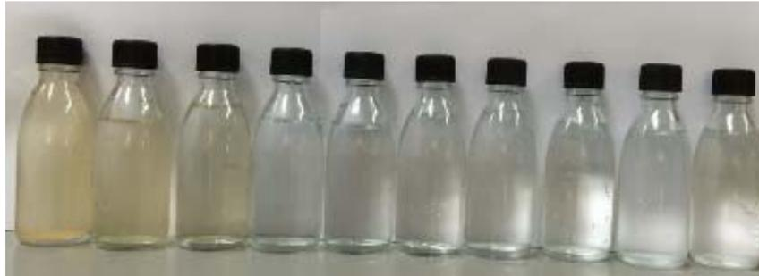
Fig. 2 – Turbidity Improvement of Chitosan Adsorption Column
