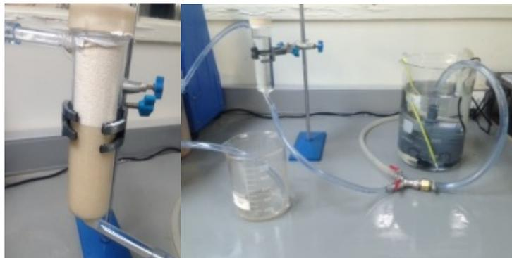
Fig. 1 – Bench Top Chitosan Adsorption
