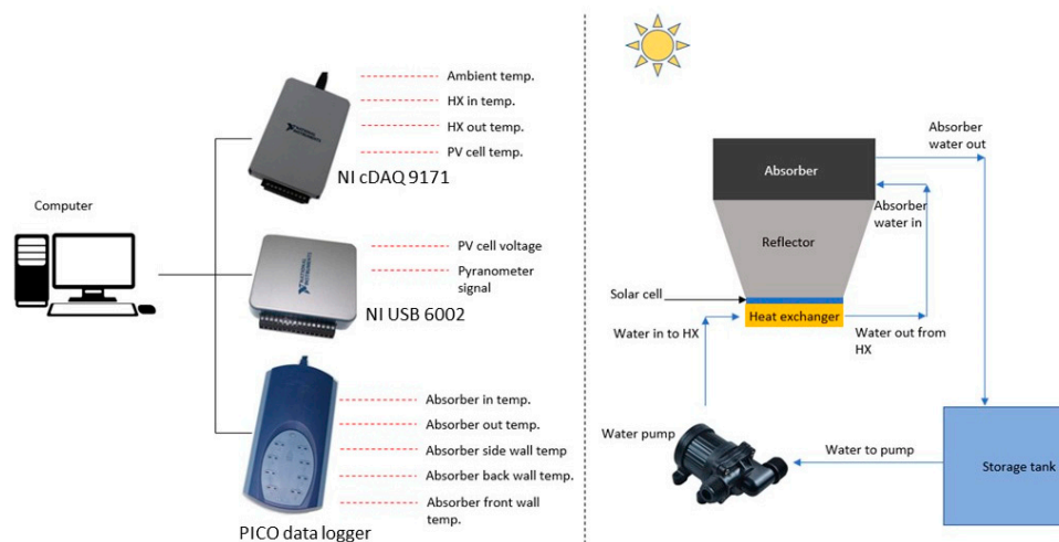
Figure 12. Left side—Depicts the instruments utilized for acquiring their respective temperature and voltage signals. Right side—Depicts the flow path of water through the module.
