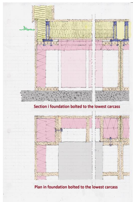
Figure 3. Foundation of fibre concrete and crawl space to access through a cover below the main door matt (Barrett, 2016).
