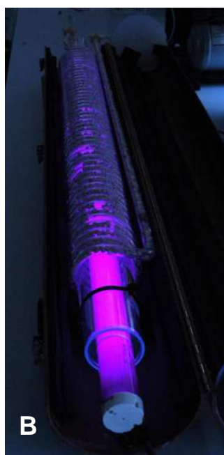
Figure 5-3. Completed photocatalytic flow reactor. (A) Compressor, reservoir and coil reactor within housing. (B) UV lamp in operation. (C) Inlet and outlet detail.
