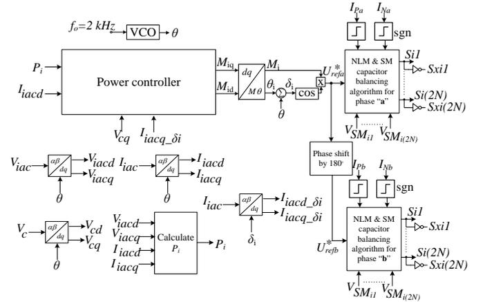
Fig. 3. Overall control structure for port  $i$ .
