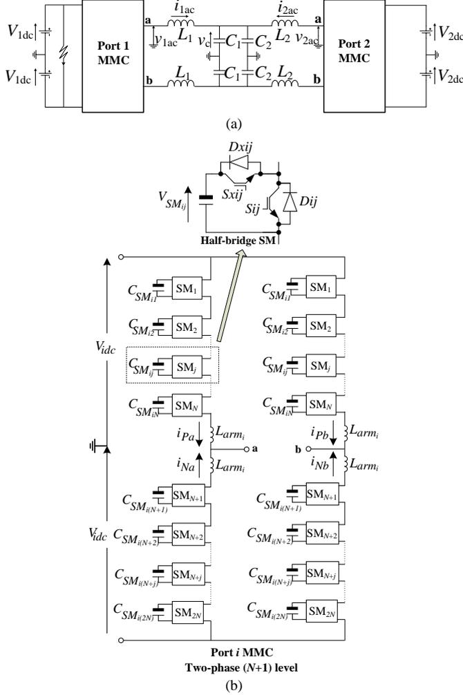
Fig. 1. Topology of MMC-based LCL DC/DC converter.
