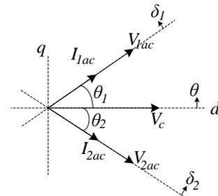
Fig. 4. DC/DC converter phasor diagram.
