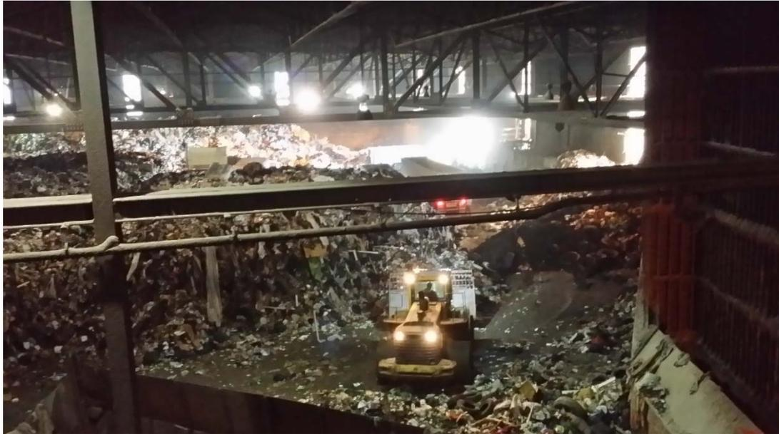
Figure 8: A Feedstock storing at the Covanta WTE plant
