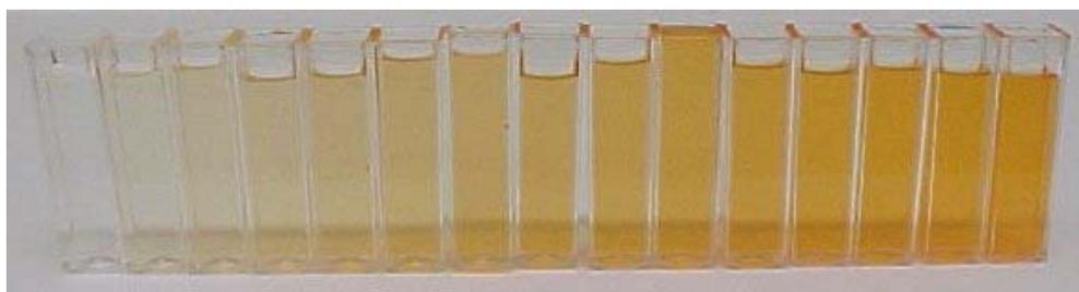
Figure 25 - Photo of the colour range of Fe-Phenanthroline from weakest (left) to strongest (right)
