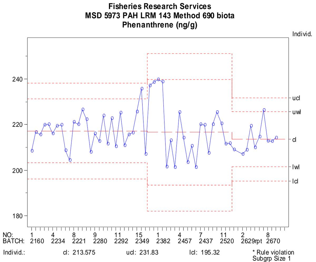
Fig. 2.1: Example of a Shewhart control chart for phenanthrene showing warning and action control limits, based on  $\pm 2 \times$  and  $\pm 3 \times$  the standard deviation of results obtained. Each data point on the plot represents a value from a single analysis of an LRM in a batch.
