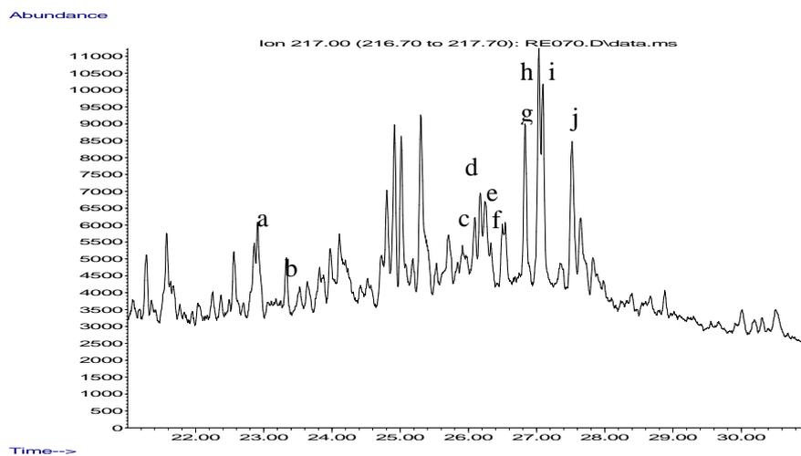
Fig. 5.5(d): Capillary column gas chromatogram of the sterane ( $m/z$  217) profile of Arabian light crude oil
