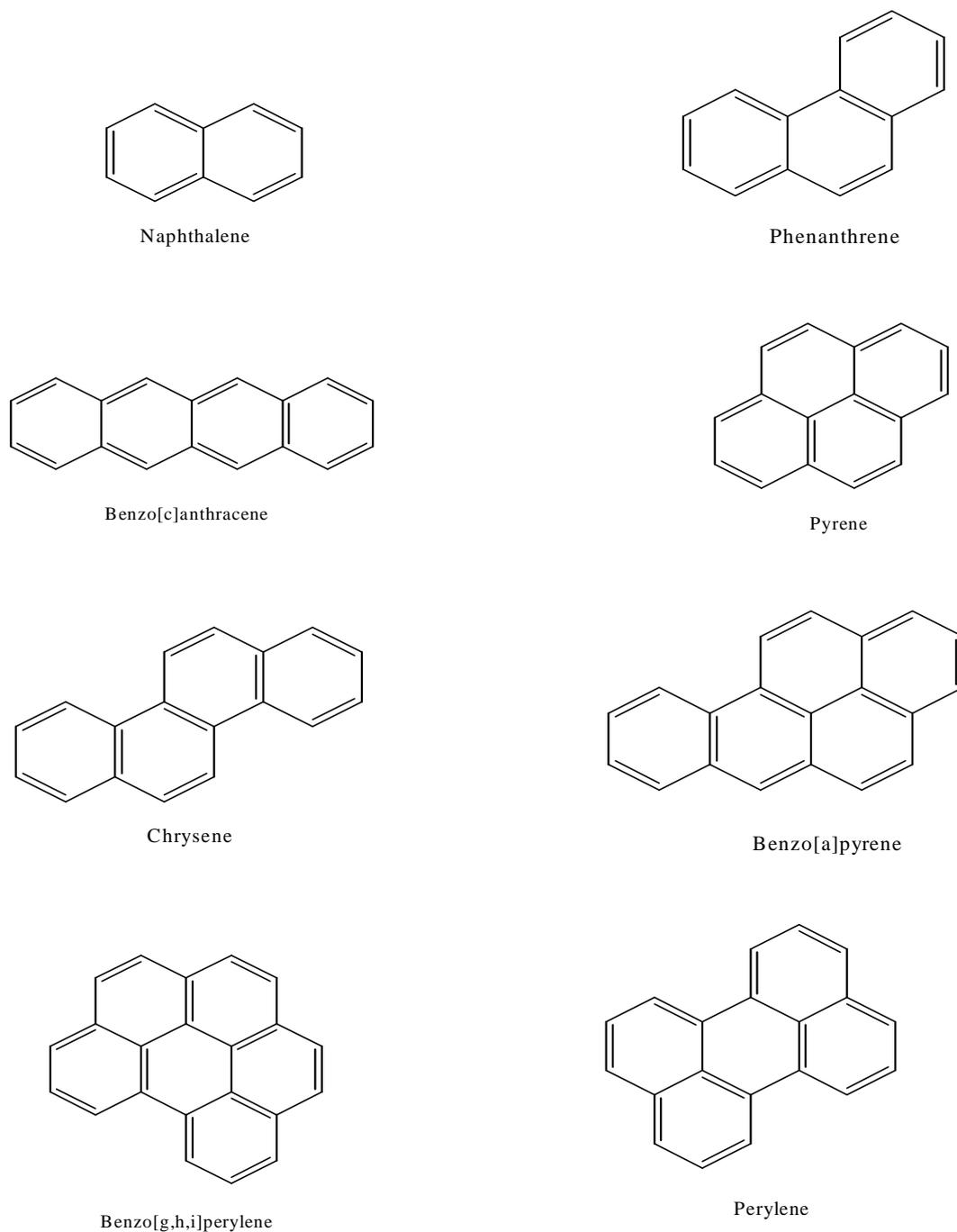
Fig. 1.2: Chemical names and structures of some common PAH compounds
