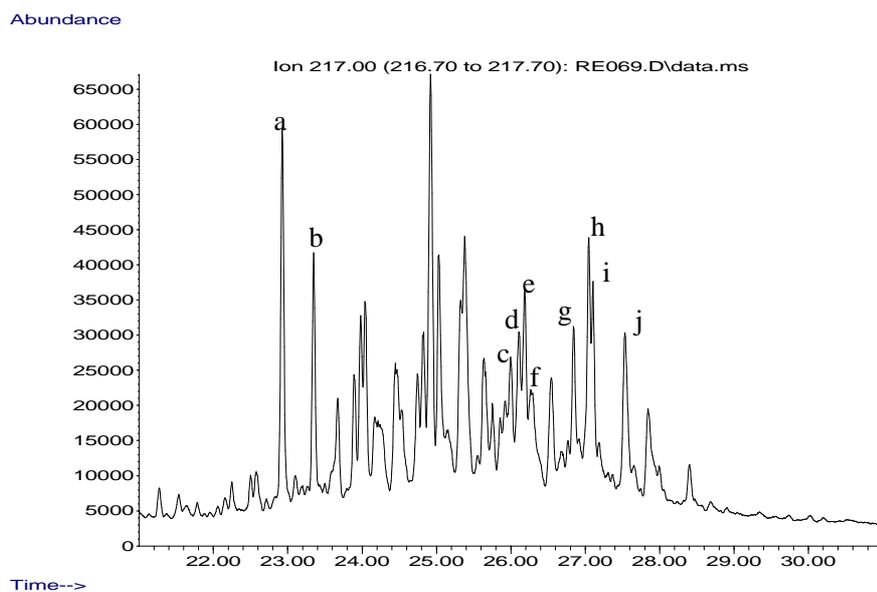
Fig. 5.5(a): Capillary column gas chromatogram of the sterane ( $m/z$  217) profile of Forties crude oil
