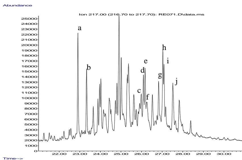
Fig. 5.5(b): Capillary column gas chromatogram of the sterane ( $m/z$  217) profile of Hutton crude oil
