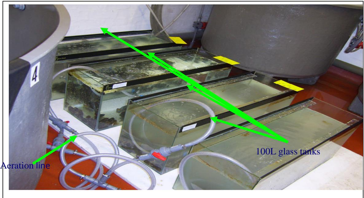
Figure 6.1: Experimental set-up showing the exposure of mussels to crude oils
