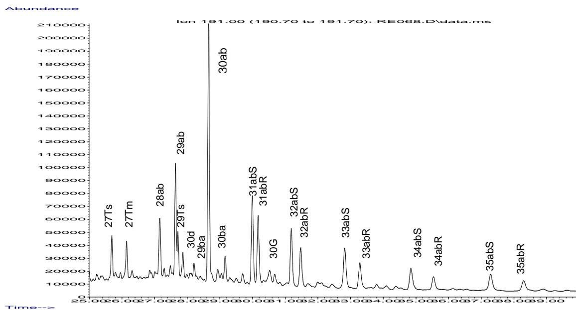
Fig. 5.2: Capillary column gas chromatogram the triterpane profile of Gulfaks crude oil.
