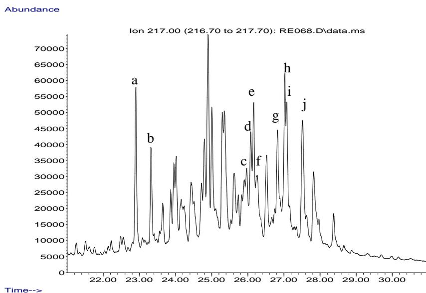
Fig. 5.5(c): Capillary column gas chromatogram of the sterane ( $m/z$  217) profile of Gulfaks crude oil
