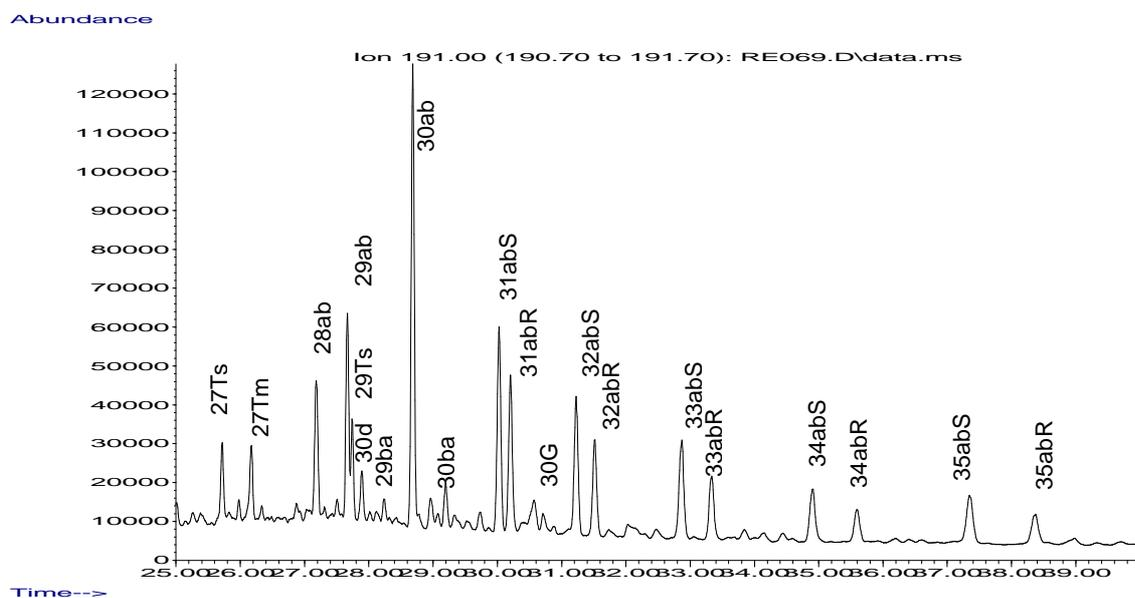
Fig. 5.1: Capillary column gas chromatogram the triterpane profile of Forties crude oil.
