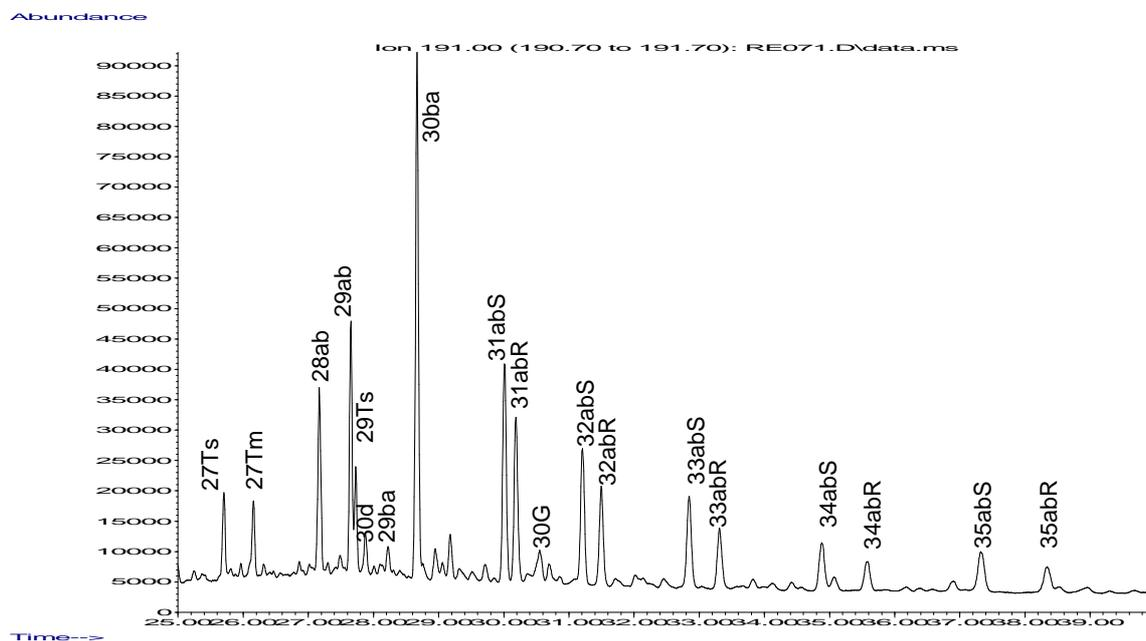
Fig. 5.3: Capillary column gas chromatogram of the triterpane profile of Hutton crude oil.
