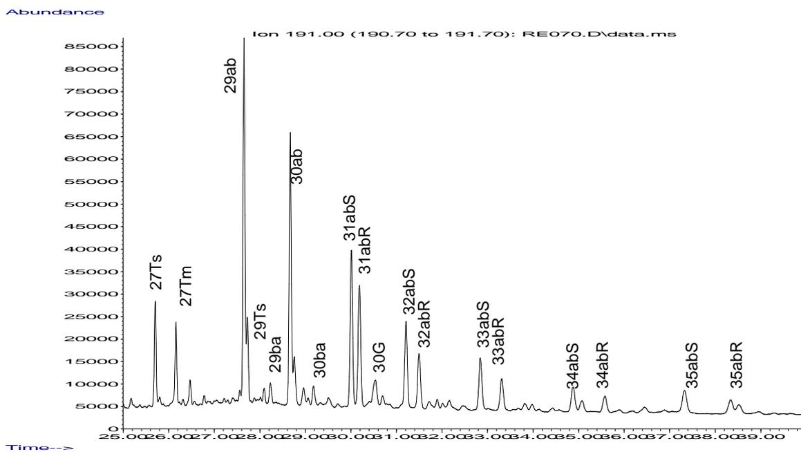
Fig. 5.4: Capillary column gas chromatogram of the triterpane profile of Arabian light crude oil.
