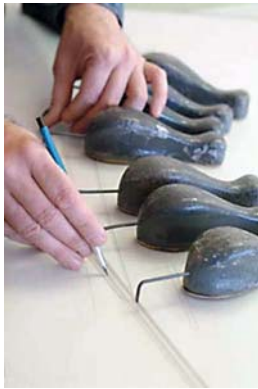
Figure 2: ‘Splines’ are long, flexible battens used in conjunction with spline weights to draw fair curves while drawing a boat’s lines and during the lofting process
