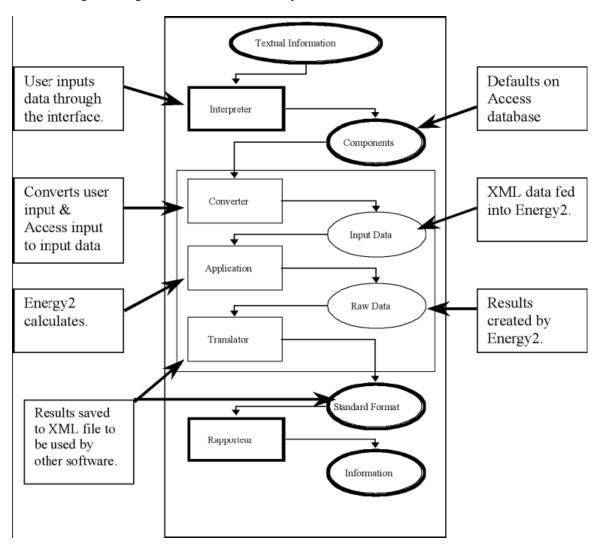
The interface between EnergySave and the application is the XML file. This Section briefly describes the system.
