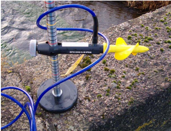
Figure 4-14: Valeport 002 Pulse counter flow meter.
