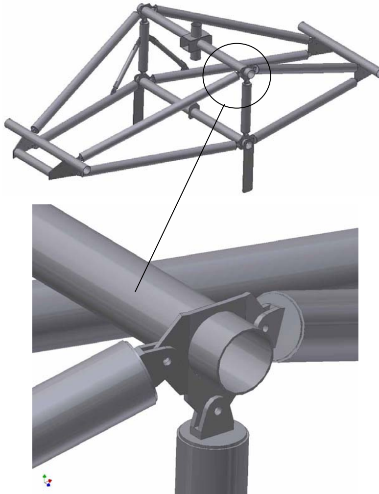
Figure 4-2: Detail of pin-jointed structure.
