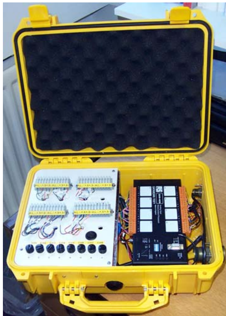
Figure 4-18: RS7221 Datascan ruggedised field unit
