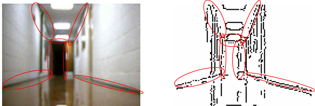
Figure 5.5 Navigation critical lines in a typical image – image1 (a) A typical image (b) Thinned version of image1
