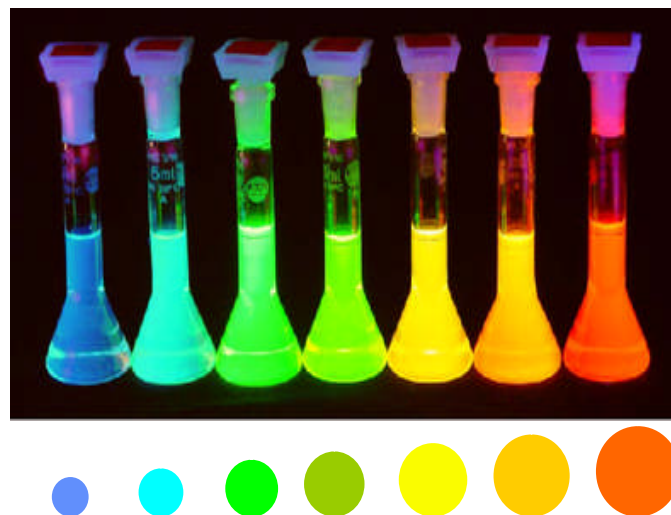
Figure 1.7 Different sized CdSe/ZnS QDs extending from 490 nm to 620 nm excited under UV light. The blue QDs dimensions are \sim 2 nm while the orange QDs measurements are \sim 6 nm 28 .
