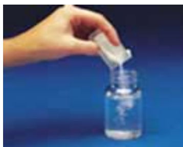
Figure 2.1 Addition of Colilert 18™ reagent to 100 ml sample of water in a sterile Colilert 18™ bottle (Reproduced with permission from IDEXX)
