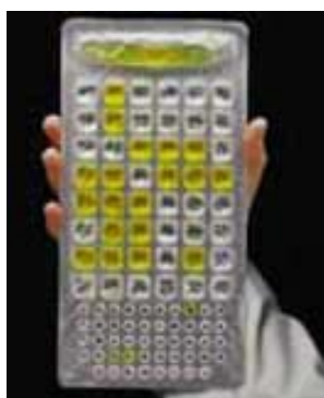
Figure 2.2: Quanti-tray™ containing water and dissolved reagent. Yellow wells indicate presence of coliform bacteria (Reproduced with permission from IDEXX)
