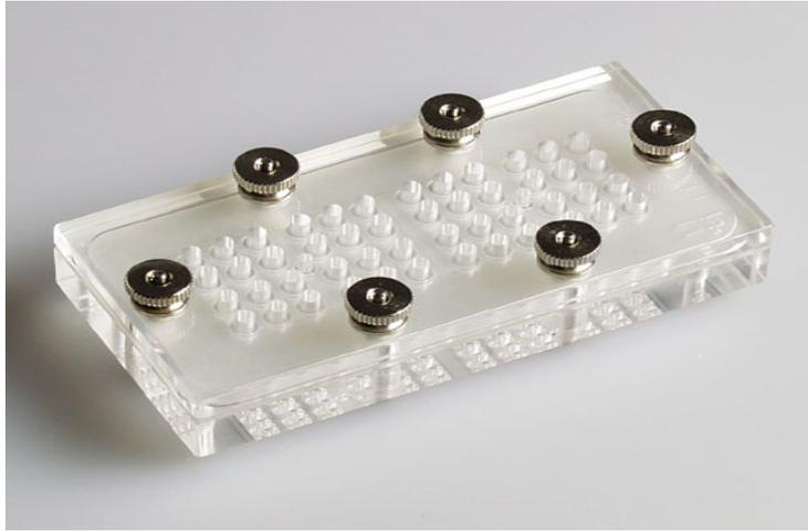
**Figure 2.5. An example of the assembled chemotaxis chamber.**
