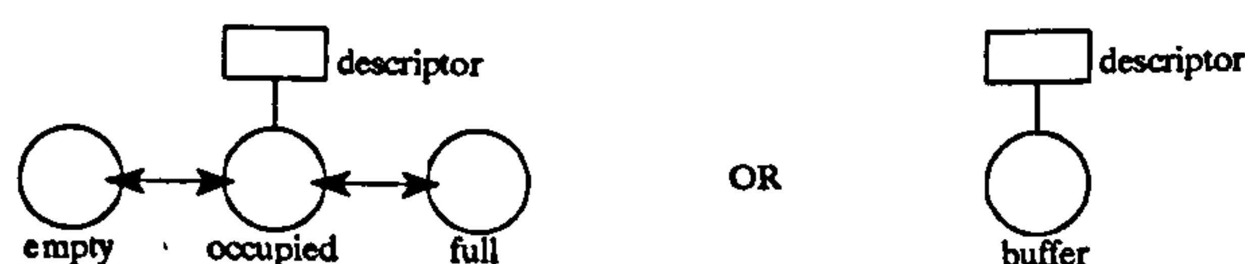
Figure 3.2 State diagram of N-place buffer using an extra descriptor
